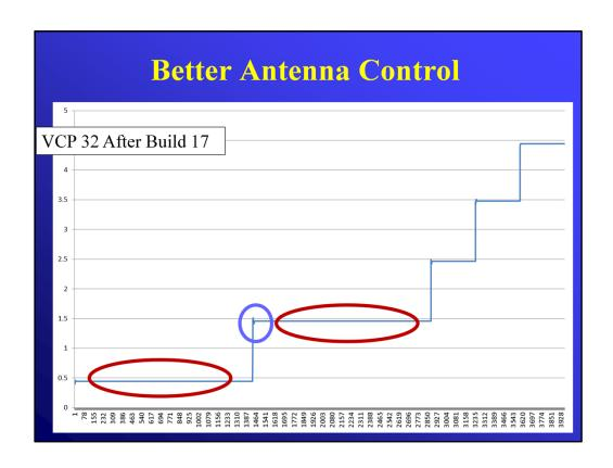
Here is VCP 32 after the installation of Build 17. There is much less wobbling when moving to a new elevation. Even more striking is the lack of dithering once the elevation has been achieved.
