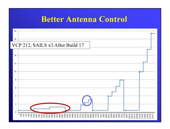
And now for VCP 212 after the installation of Build 17. Just as with VCP 32, there is much less wobbling when moving to a new elevation, and the antenna is much more stable while the data at an elevation are collected.
