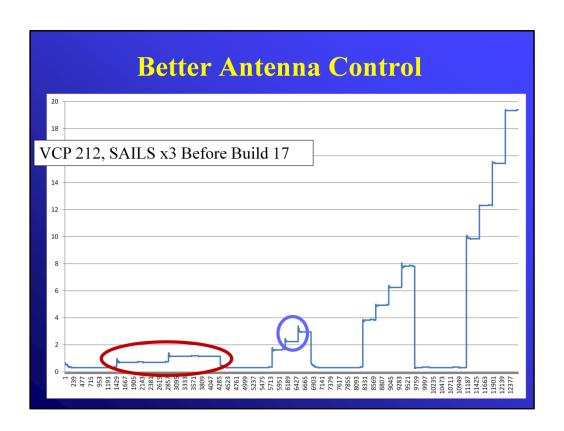
Here is a similar example for VCP 212, with SAILS x3, before the installation of Build 17. You can see the three times that the antenna drops down to collect the SAILS cut data. The purple circle shows us the most obvious wobble at the beginning of an elevation, and this exists throughout the volume scan. There is also dithering highlighted by the red oval for the two elevation where it's easiest to see.
