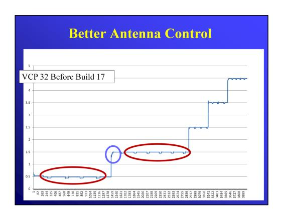
Here's an example from one of the Build 17 Beta sites. Before the installation of Build 17, this graphic shows you the antenna position for VCP 32. The purple circle shows us one of the transitions to a new elevation, which has some "bumps" in it. The red ovals show what is called "dithering" as the data are being collected. Dithering is occurring on all of the elevations.
