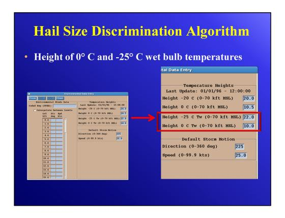
To support the Hail Size Discrimination Algorithm, it is important to keep the heights of the 0° and -25° C wet bulb temperatures current in the Environmental Data at the RPG. These values will be computed from the existing environmental model data received from AWIPS. As with other environmental data, it is recommended that these wet bulb temperature heights be checked periodically for quality control.
