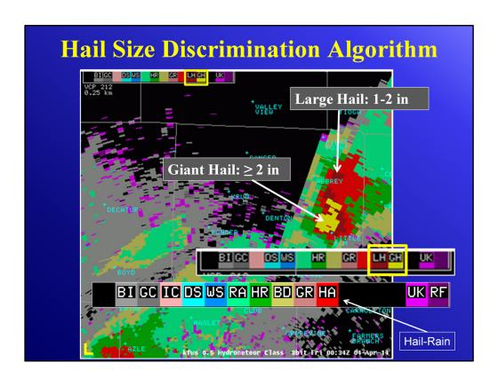
Here's a closer look at these new hail classifications. This is an HCA product at 0.5° elevation, and the storm is at a far enough range to sample the hail core. At the bottom of the slide is a close up of the legend without the new hail hydroclasses. The bright red is "hail possibly mixed with rain", the only hail hydroclass before Build 17.0. With HSDA, the two new hail hydroclasses are in dark red for Large Hail (LH) and Yellow for Giant Hail (GH).
