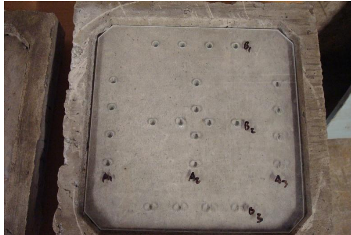
Figure 4.10 - Wenner Probe Grid
