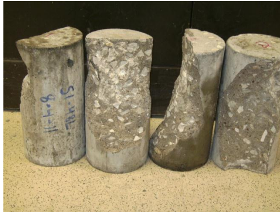
Figure 3.2 - High Strength Compressive Strength Specimens Post-Test
