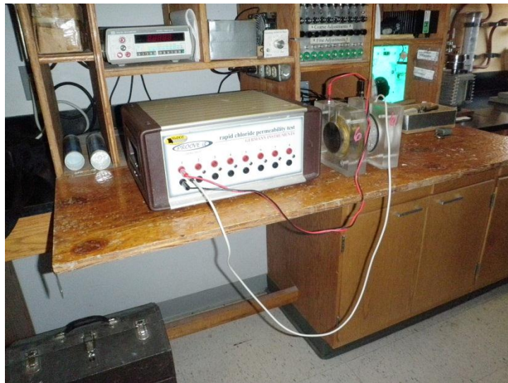
Figure 2.10 - Typical RCT Setup
