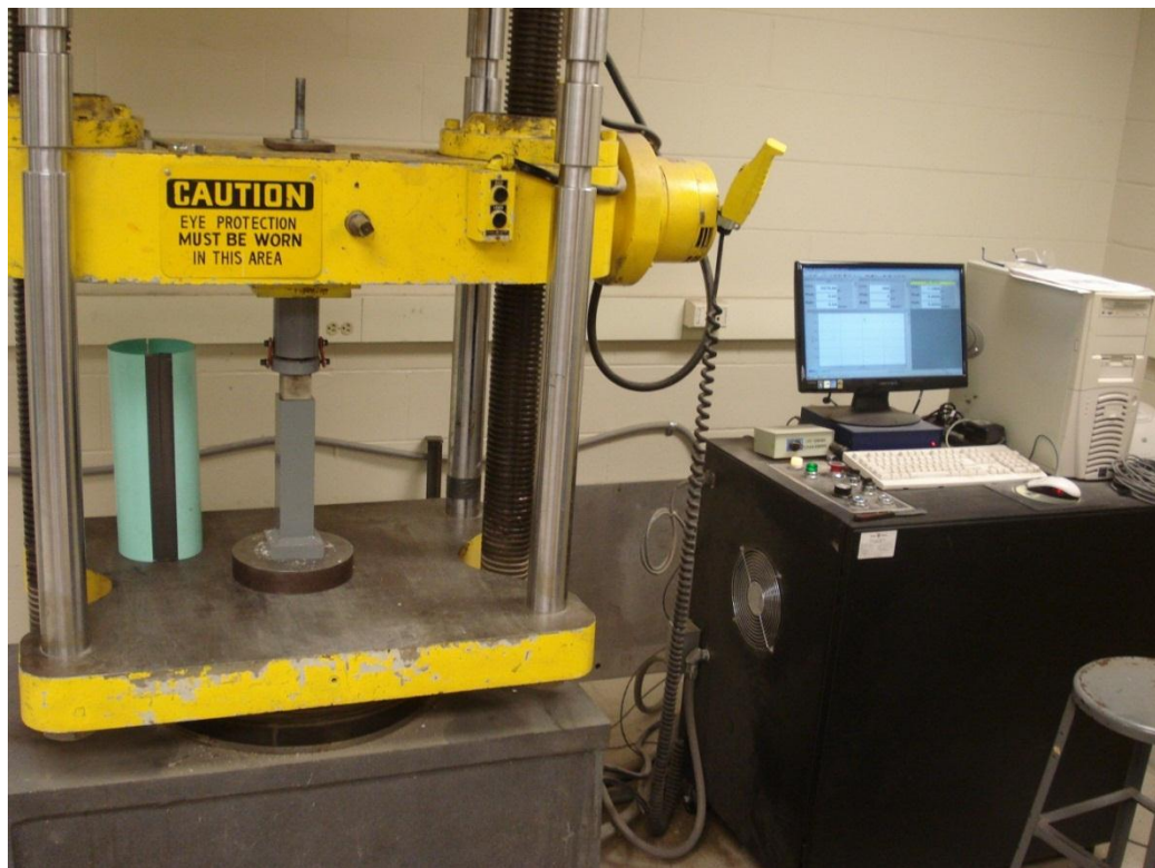
Figure 4.5 – Tinius-Olsen load frame and computer
