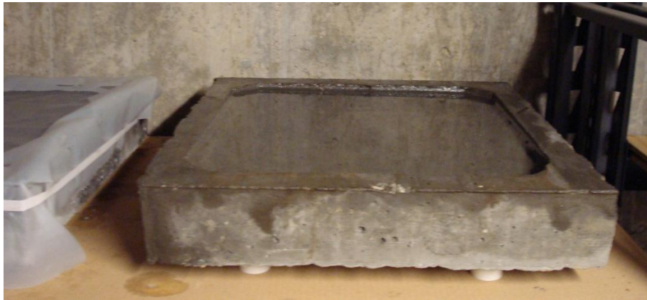
Figure 4.6 - Typical Ponding Specimen
