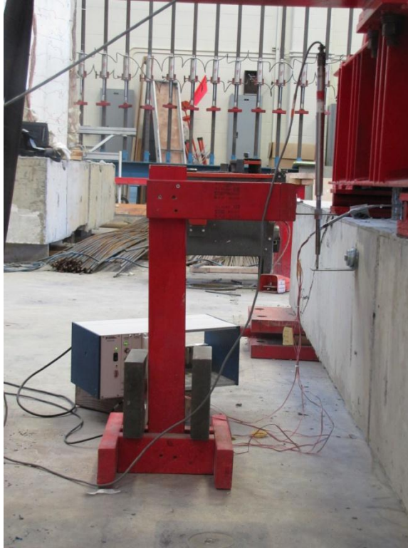
Figure 4.11- Detail of LVDT for Deflection Measurement
