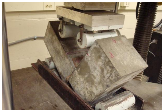
Figure 3.7 - Modulus of Rupture Specimen Post-Test
