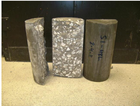
Figure 3.10 - Splitting Tensile Specimens Post-Test
