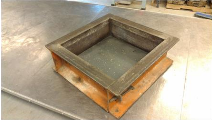
Figure 5.10 – Salt Scaling Mold
