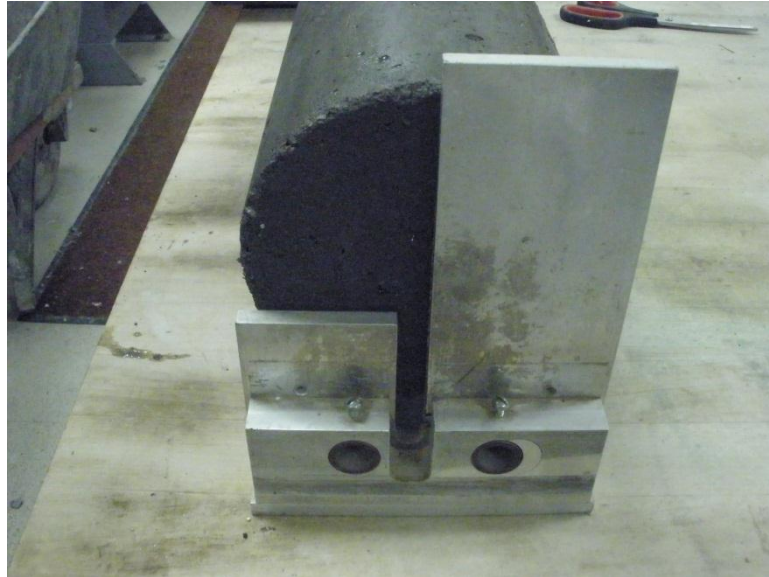
Figure 5.5 - Cylinder Marking Jig
