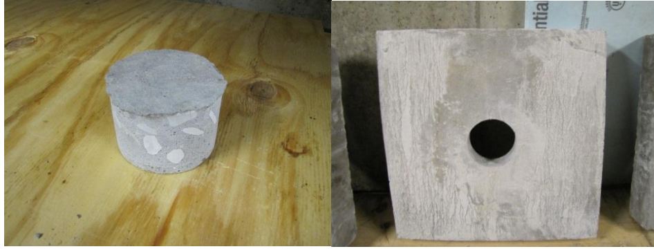
Figure 4.7 - Concrete Core and Resulting Void in the Concrete Specimen
