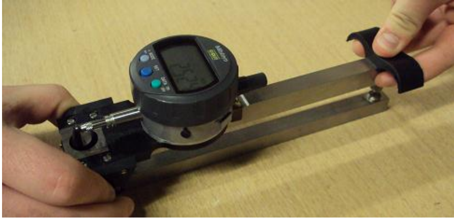
Figure 2.5 - Reading Taken on Reference Bar
