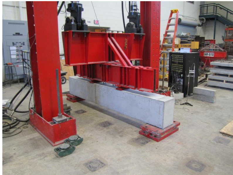
Figure 4.16 – Beam positioned within load frame
