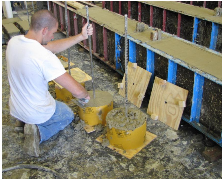
Figure 4.3 – Pull-out specimen construction
