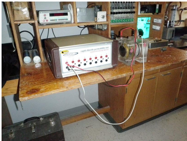
Figure 4.5 – Typical RCT Setup
