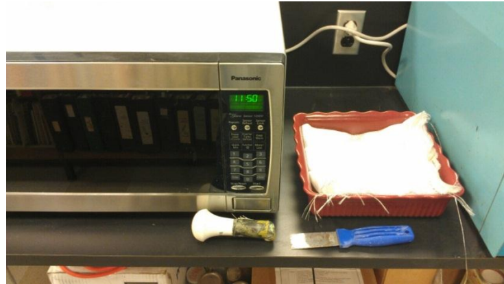
Figure 5.2 - Microwave Water Content Station
