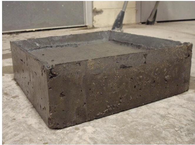
Figure 4.13 - Completed Scaling Specimen and Dike
