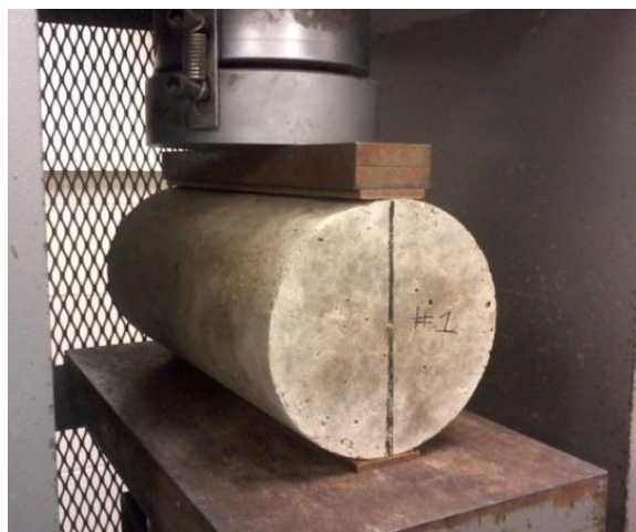
Figure 3.9 - Typical Splitting Tensile Test Setup
