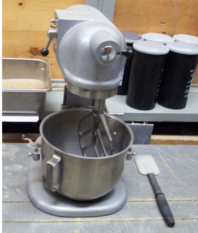
Figure 4.12 – Hobart mixer with bowl scraper
