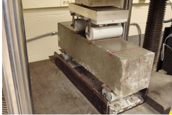
Figure 3.6 - Modulus of Rupture Testing Setup
