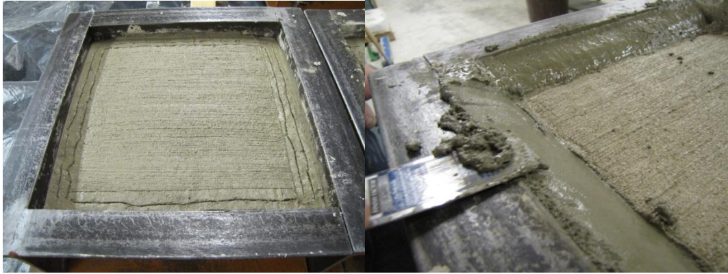
Figure 4.12 - Scaling Specimen Dike Keyway and Dike Construction
