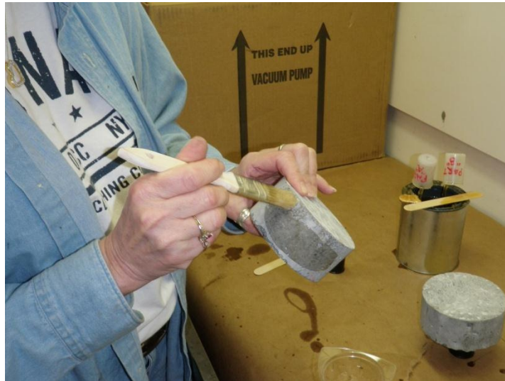
Figure 4.3 - Setting Coating Being Applied to Concrete Specimens
