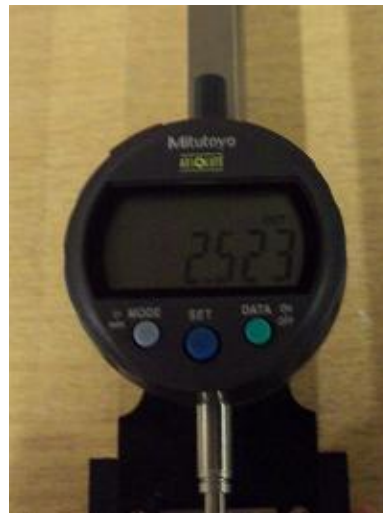
Figure 2.7 - Example DEMEC Gauge Reading
