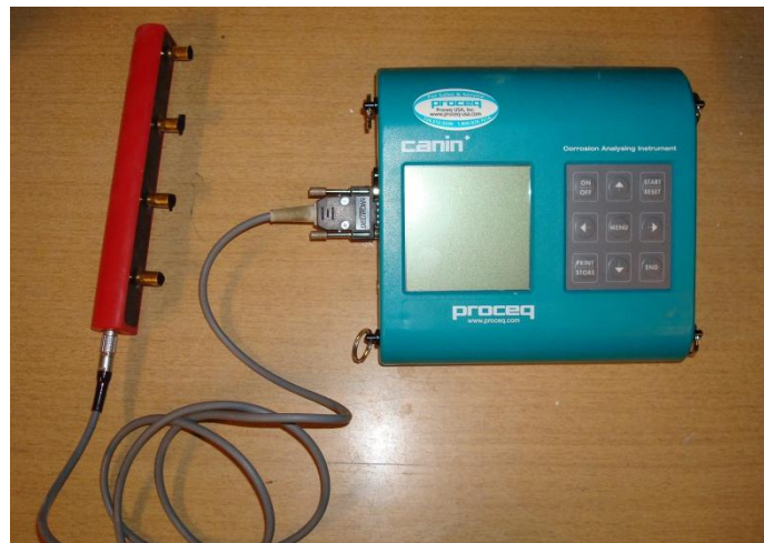
Figure 4.9 - Canin + Wenner Probe
