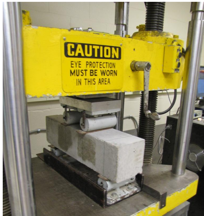
Figure 3.5 – Modulus of rupture test setup
