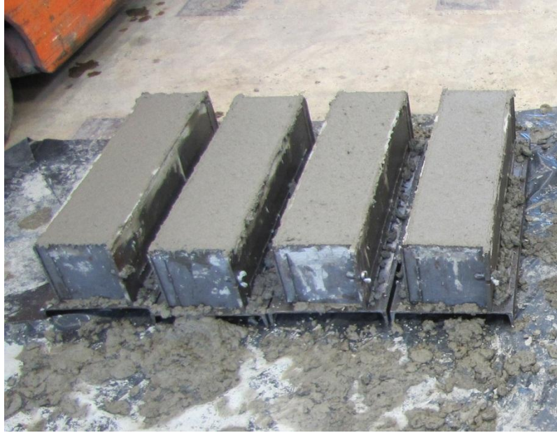
Figure 3.4 – Modulus of rupture test specimens
