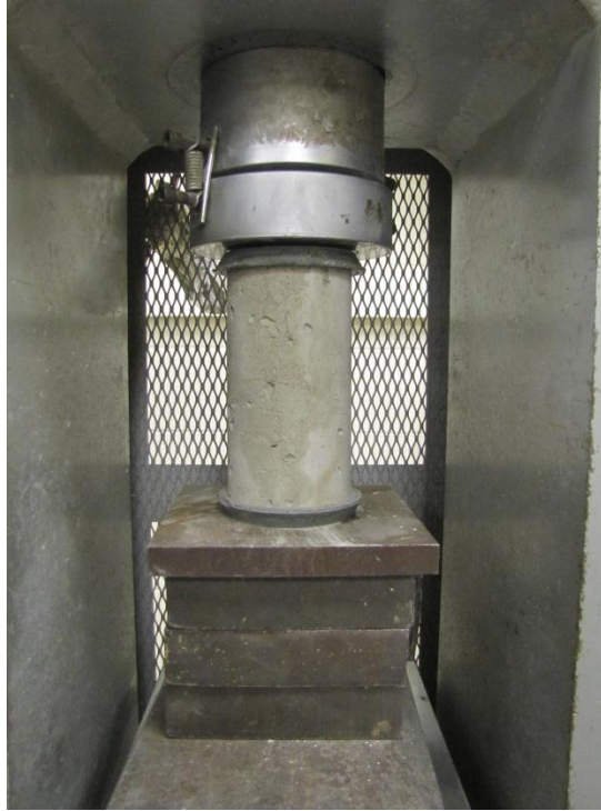
Figure 3.1 - Compressive Strength Testing Setup
