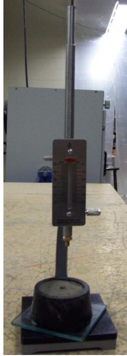
Figure 4.11 – Vicat apparatus with ring and glass plate
