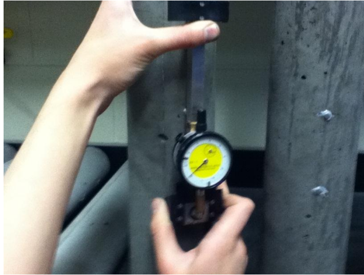
Figure 5.9 - DEMEC Gauge and Specimen
