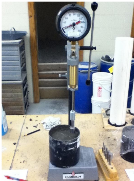
Figure 5.3 - Concrete Time of Set Equipment
