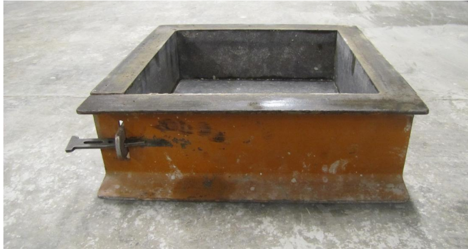
Figure 4.11 - Scaling Specimen Form
