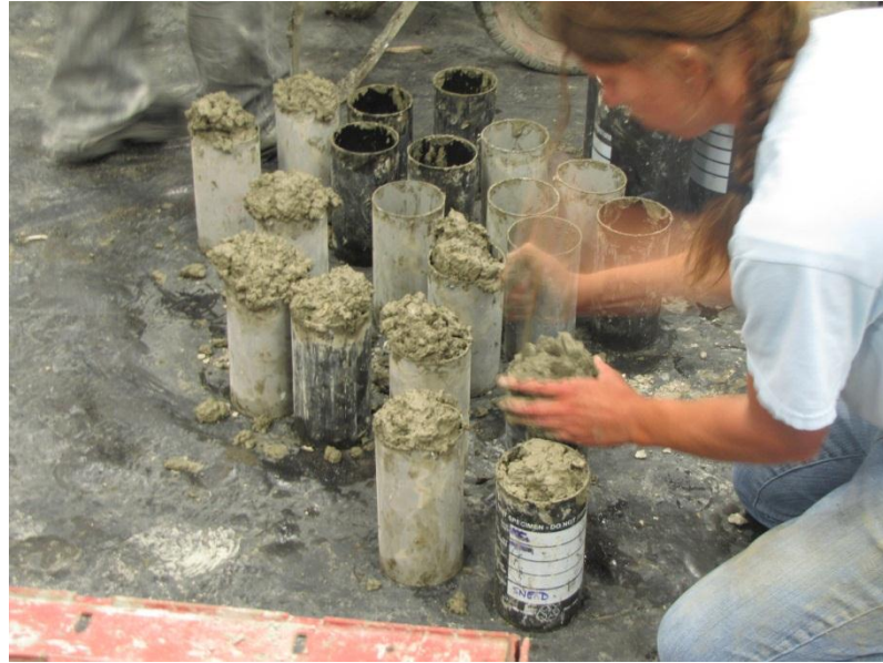
Figure 3.2 – Casting compressive strength cylinders
