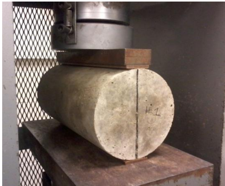
Figure 3.6 – Splitting tensile strength test setup
