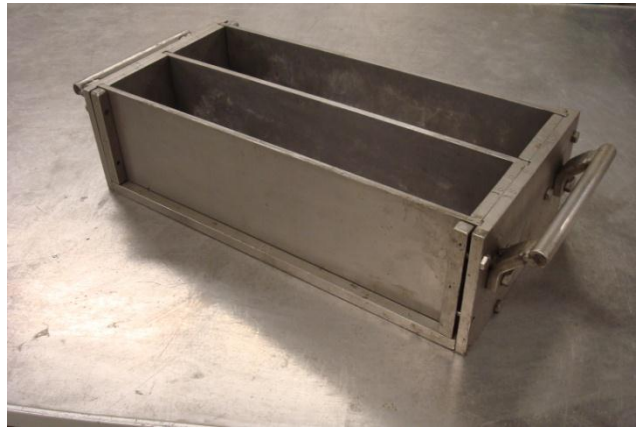
Figure 4.1 - Freezing and Thawing Specimen Molds
