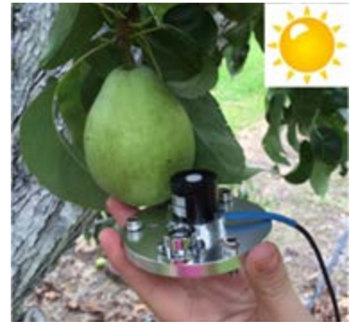
Figure 3: Measurement of PAR of an internal fruit (<30% light interception) using the Q53292 quantum sensor (Licor). .
