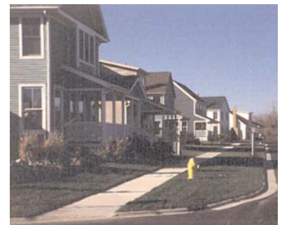
Figure 24. Photograph shows reduction in front yard setback to reduce amount of impervious surface in service sidewalks and driveways.
