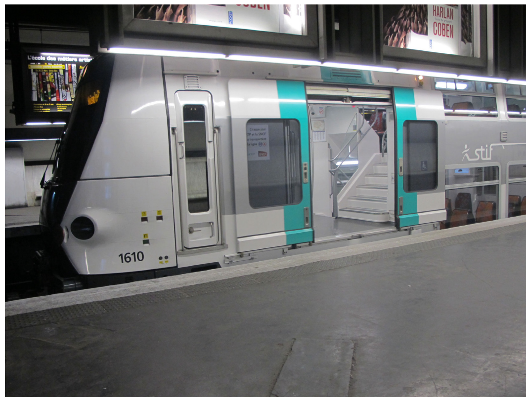
Figure 9: The MI-09 is a double-deck, dual-voltage electric multiple unit trainset that is operated on RER A, a hybrid suburban commuter and rapid transit system serving Paris and its Île-de-France suburbs.
