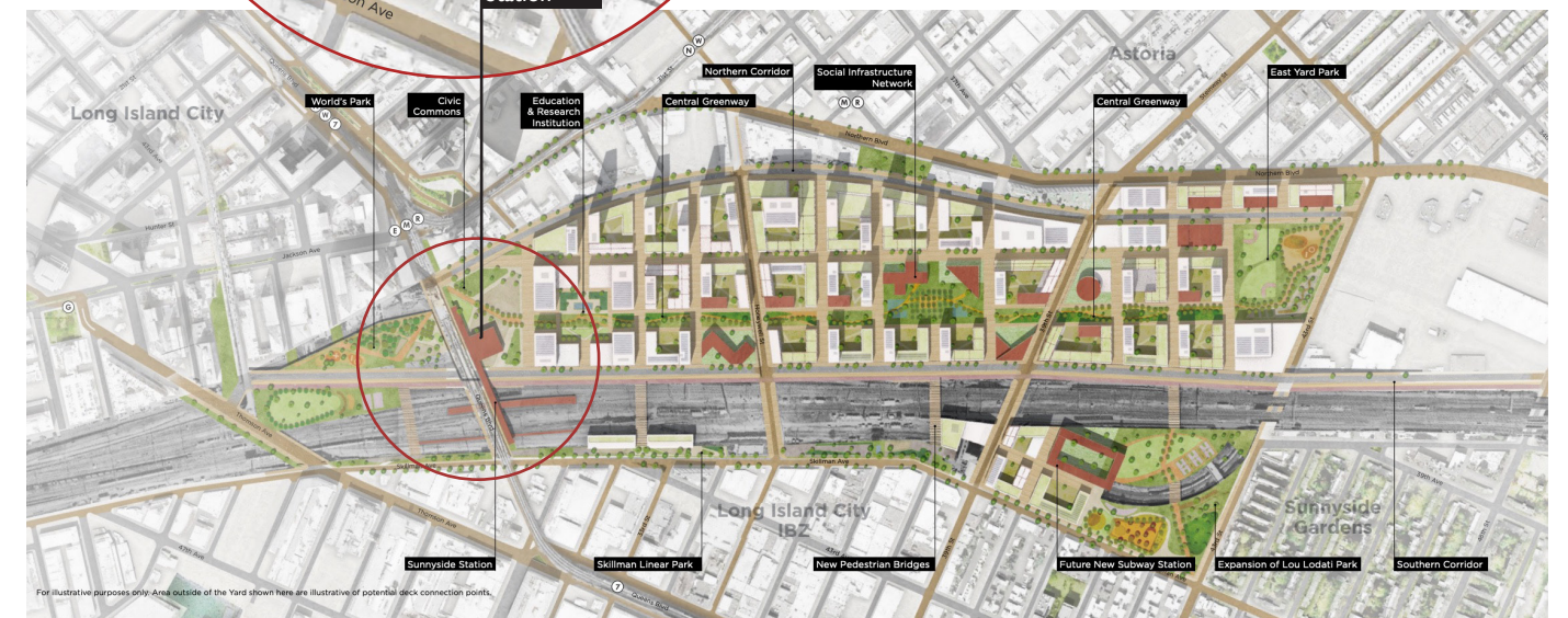
Figure 24: The NYCEDC Sunnyside Yard Master Plan includes a small two-platform station for LIRR service. Under a through-running scheme, the Sunnyside Station will require a larger footprint to handle NJT and MNR service.
