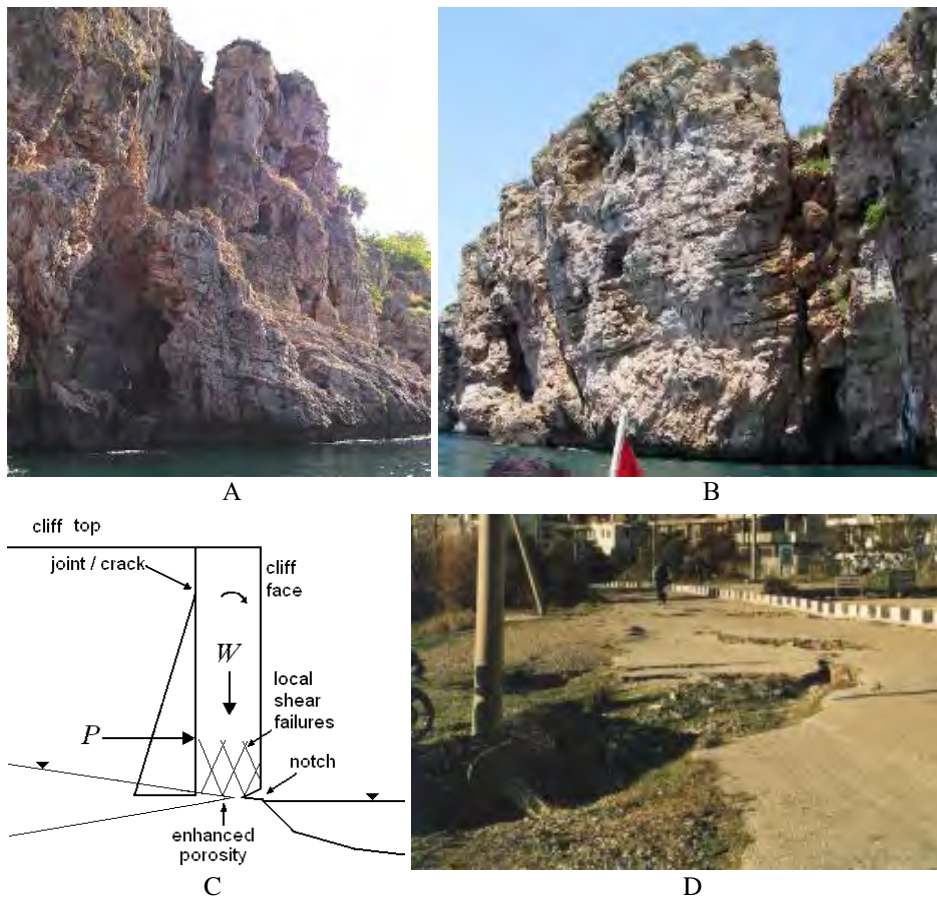
Figure 18. A-B) Tilted blocks on the cliff, C) Permanent residual tilt as a result of water pressure, D) Tilt of blocks and deformations on the cliff top after heavy and long duration rainfall.
