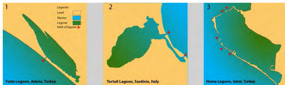
Figure 1. Lagoon systems; 1. Choked, 2. Restricted, 3. Leaky (redrawn from Kjervfe, 1994).
