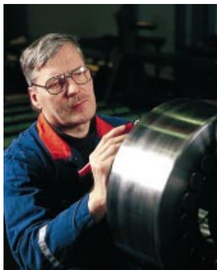
Esa Isometsä is checking the roundness of a Sendzimir mill's support bearing at the Tornio cold rolling plant.
