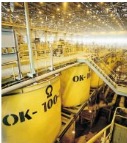
Outokumpu is the market leader in flotation technology. A record number of Outokumpu flotation cells were sold in 1996, most of them to South America. Pictured are thirty-two OK-100-TC tank cells waiting for installation at Codelco's Andina mine (above) and the Escondida mine's concentrator (below), both in Chile.
