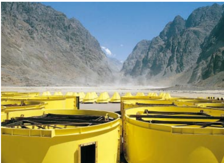
Outokumpu is the market leader in flotation technology. A record number of Outokumpu flotation cells were sold in 1996, most of them to South America. Pictured are thirty-two OK-100-TC tank cells waiting for installation at Codelco's Andina mine (above) and the Escondida mine's concentrator (below), both in Chile.
