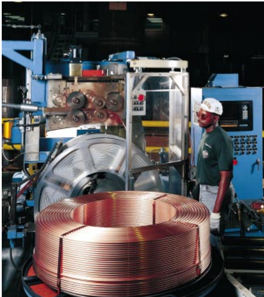
Outokumpu produces demanding tubes for the air-conditioning industry in Franklin, Kentucky, the United States. The tubes' heat transfer area is increased by sophisticated enhancements on the interior surface. This technology has been developed by Outokumpu. Doug Holder is operating a level winder.
