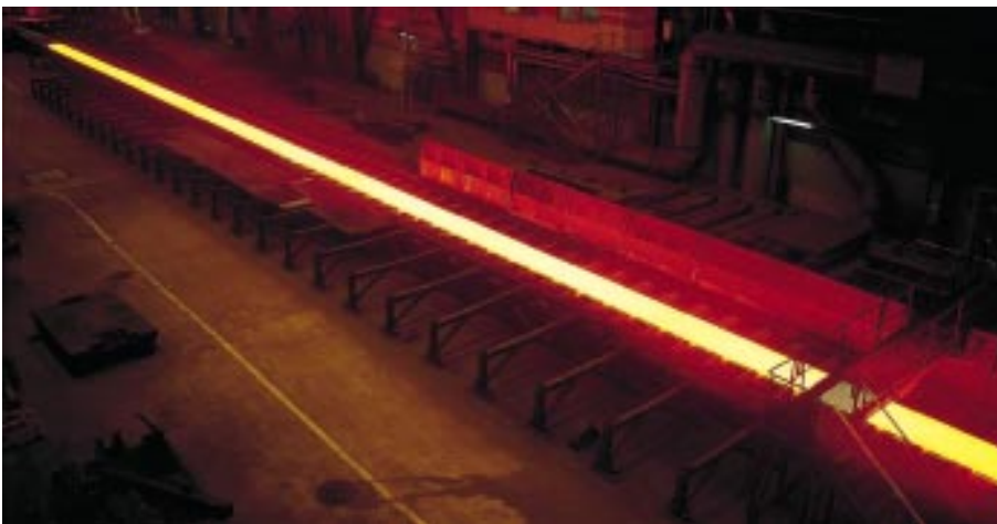
The most spectacular phase of stainless steel production is hot rolling. A steel slab is rolled down to 8 mm's thickness, after which it moves to the down coiler.
