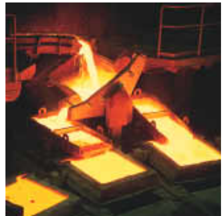
Harjavalta produces blister copper with a copper content of 99.2%. In the picture copper is cast into anodes to be delivered mainly to the Pori tankhouse for electrolytic refining.
