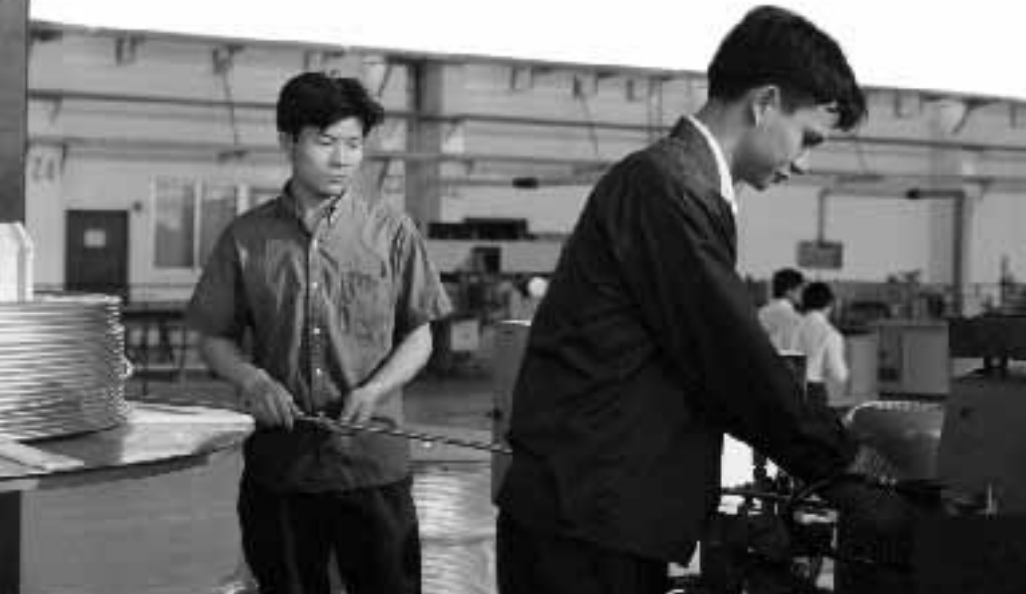
Outokumpu's technological expertise has been transferred close to customers, e.g. to the Chinese copper tube plant, that manufactures demanding, inner-grooved air-conditioning tubes. Pictured are Chen Young (right) and Liang Laian coiling tube.
