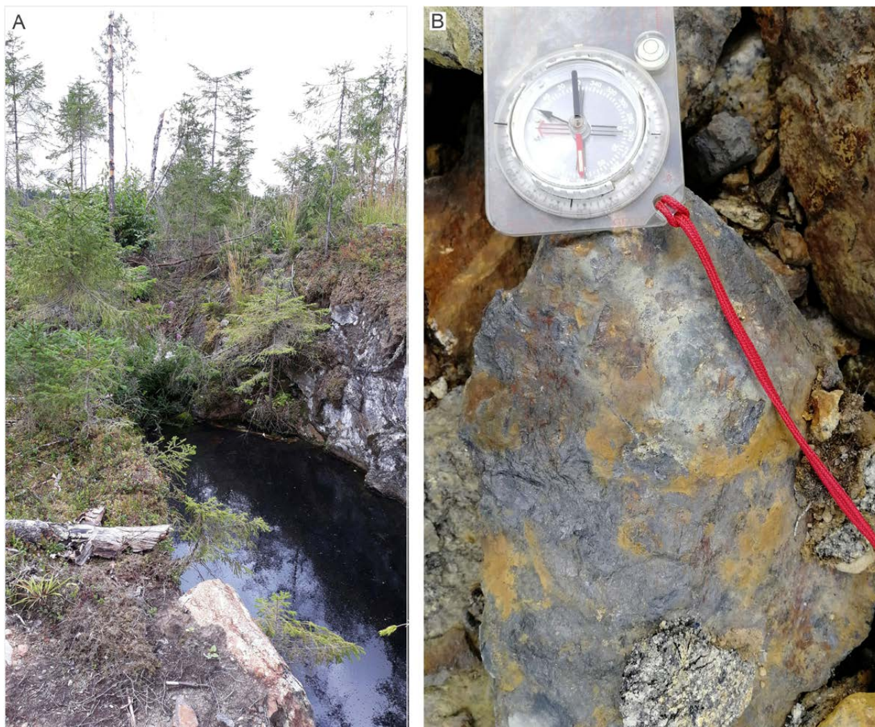
Fig. 62. A) Historic graphite mine in Haapamäki, width of the mined exceptionally rich graphite layer was less than 5 metres. B) Ore from the Haapamäki mine, width of compass 6 cm.
