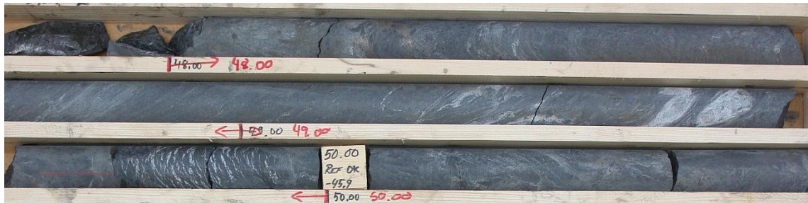
Fig. 14. Drillhole R15. 10.4 % graphite at 49-50 m.
