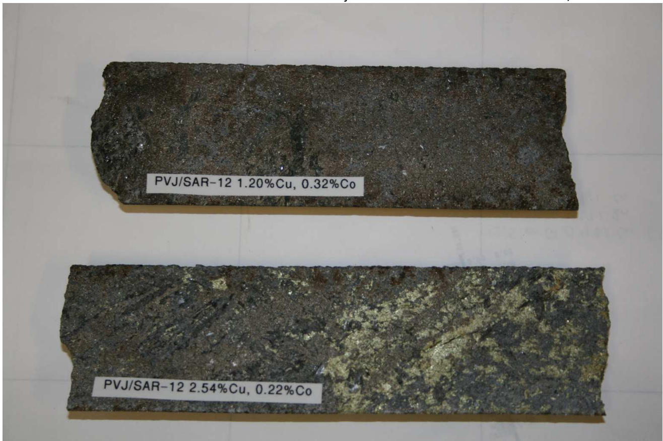
Figure 13. Samples of Saramäki pyrrhotite-chalcopyrite mineralised tremolite-chlorite-carbonate skarns. Samples PVJ/SAR-12/73.07m (up) and PVJ/SAR-12/74.97m (below).
