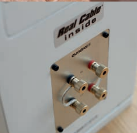
Bi-Wiring-Terminal Area with an elaborated cable bridge
