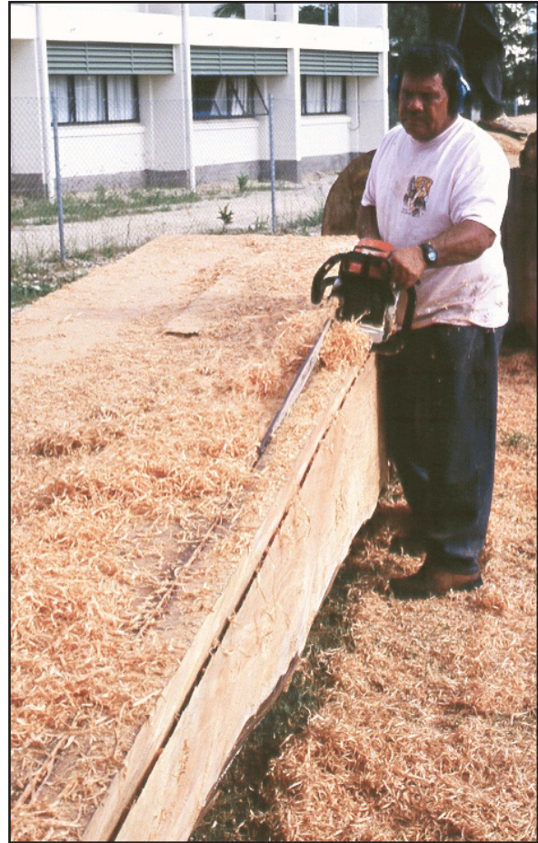
Figure 52. Rough cut of hull thickness was made for entire length of a hull segment.
