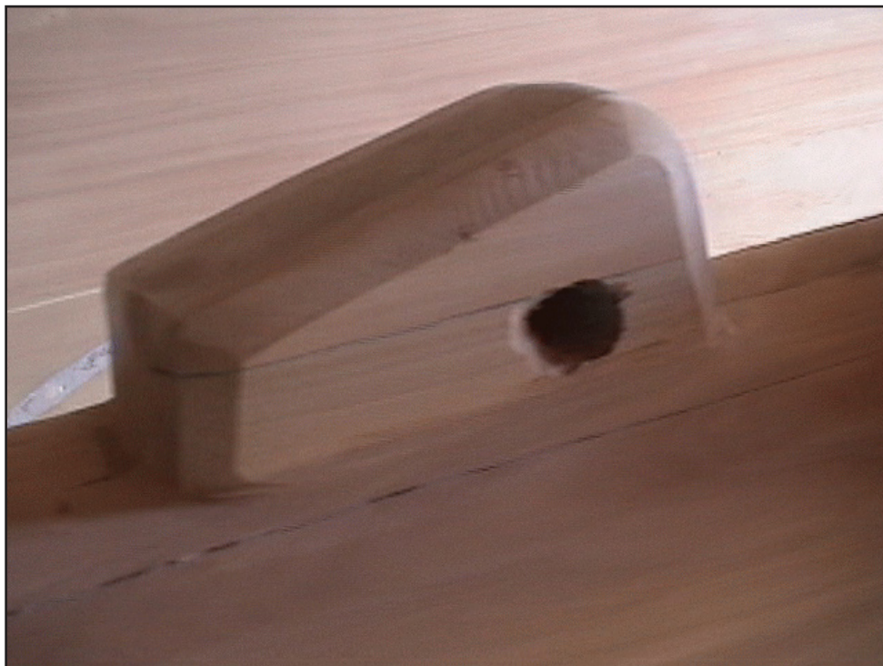
Figure 128. Cleat on the side of the mast for use in tying on the shrouds.
