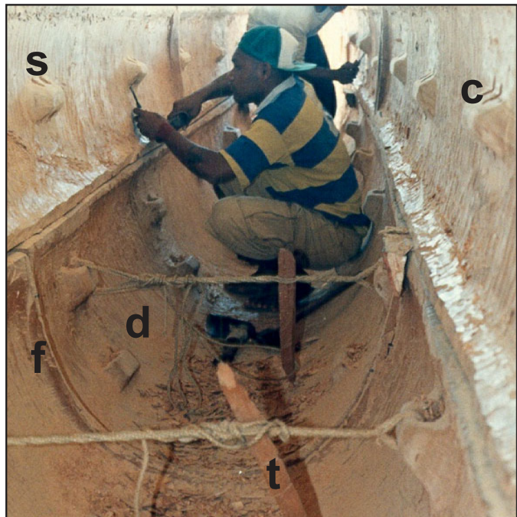
Figure 65. Finishing touches were made on the comb cleats (c). Notice the flanges (f) or thick lips where dugout hull segments (d) and strakes (s) met. Also note the tourniquet style ropes (t) between hull bottom comb cleats which were used to temporarily reinforce sides while placing strakes above.
