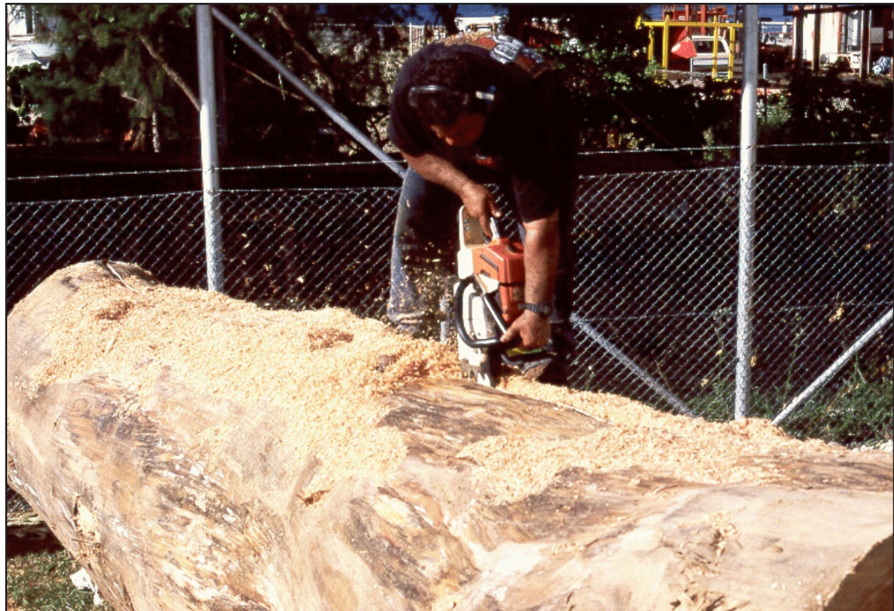
Figure 41. Log halves to be used for the dugout segments of the hull's bottom.
