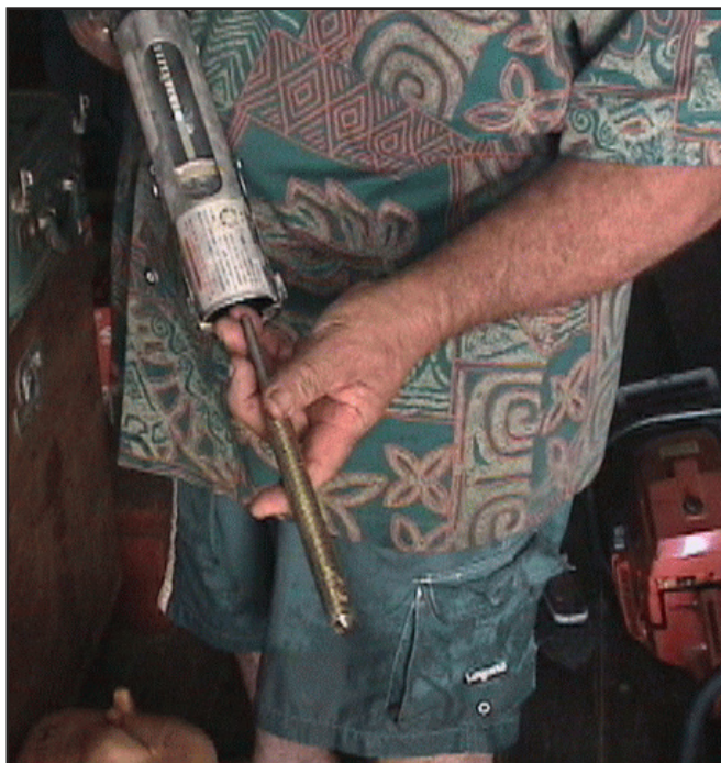
Figure 78. Glue gun used to insert glue into the metal dowels end of the metal dowels.
