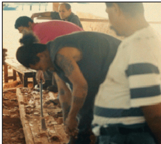
Figure 71. The strake was hollowed out. Comb cleats were left built in.
