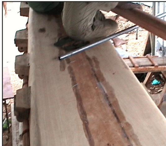
Figure 101. View of the prow shows the positioning of the yard rail in relation to the runners.
