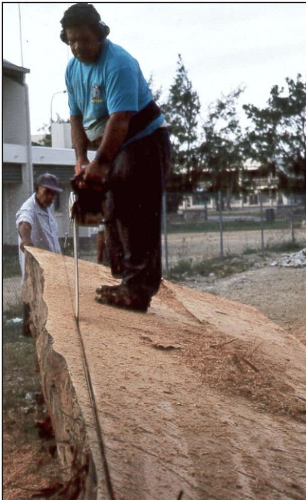
Figure 47. The log half was squared by cutting to the log's narrowest width.
