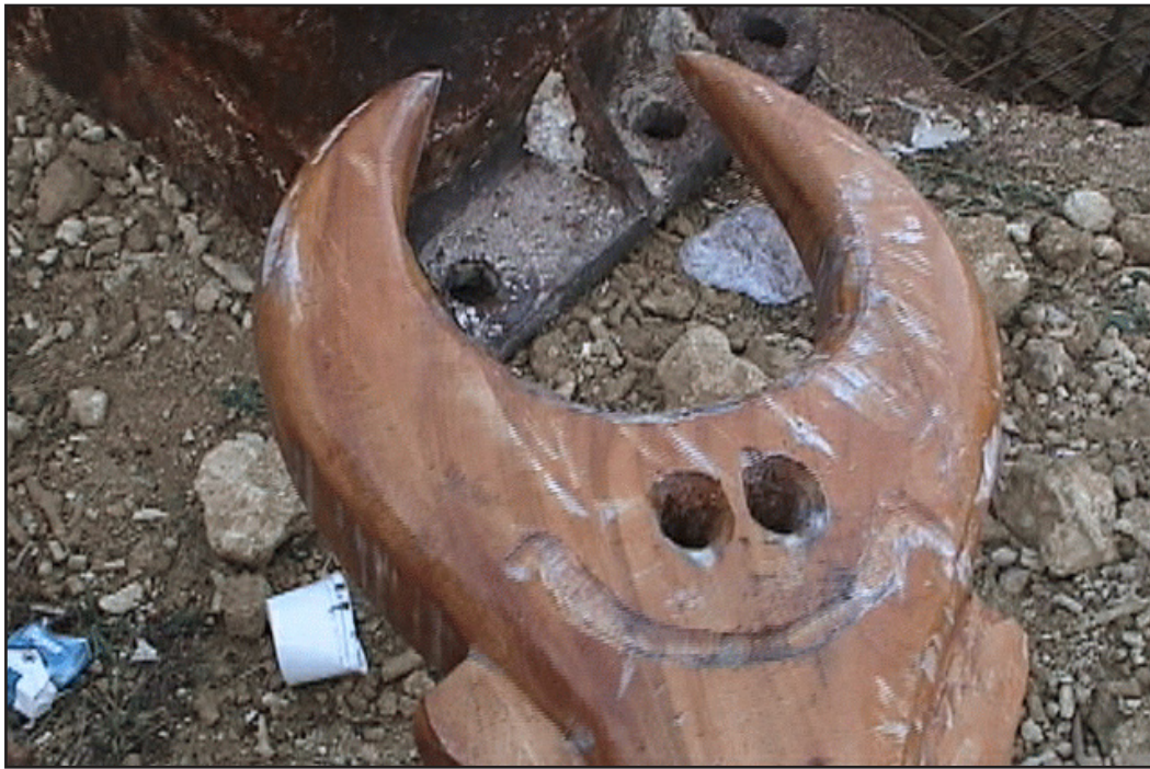
Figure 129. Claw of the small kalia mast.
