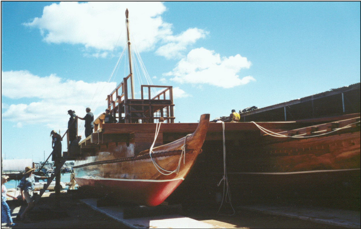
Figure 144. Here can be seen one mast which was raised and the hulls with their bottom paint and waterline painted on.
