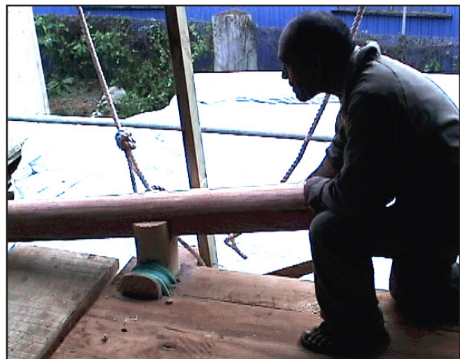
Figure 99. The first yard rail was placed from the tip of the prow to the deck.
