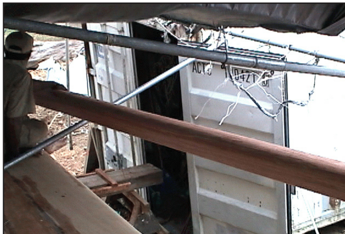
Figure 100. The yard rail ran along the leeward side of the katea .
