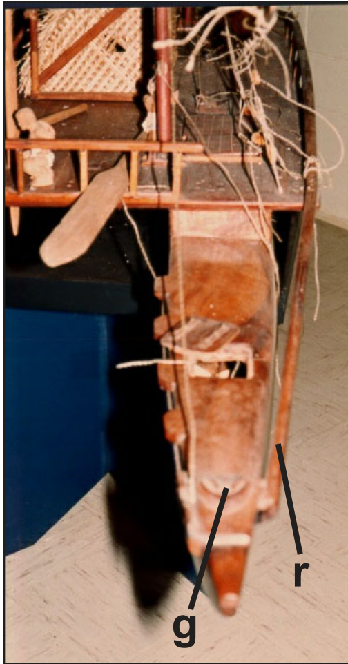
Figure 13. When the yard foot is popped out of the groove (g), it is then slid along the yard rail (r) which can be seen on the right side of this model.
