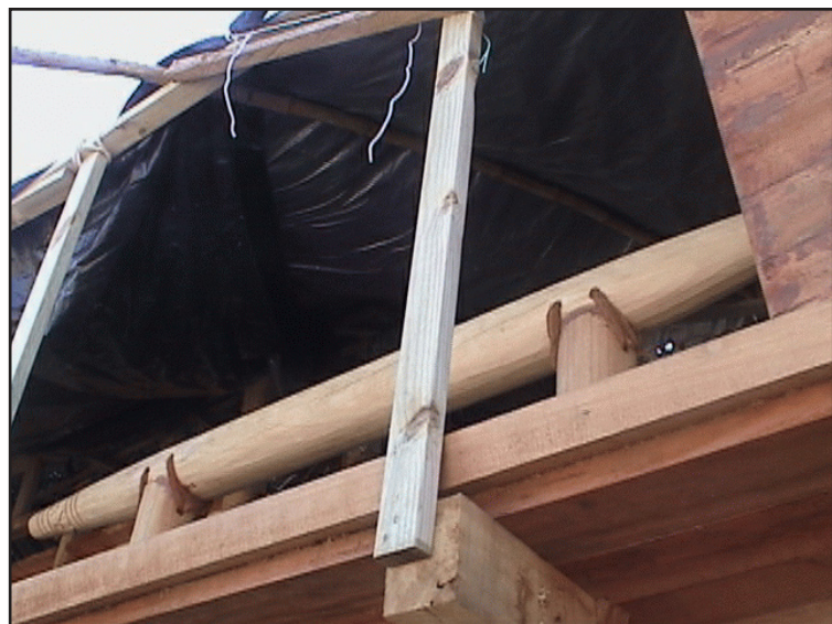
Figure 124. Large cleat on windward side of the hama , one for each mast. Its purpose is to prop the shroud which is tied to the crossboom on this side over the fale so there is no obstruction to the shroud when under sail.
