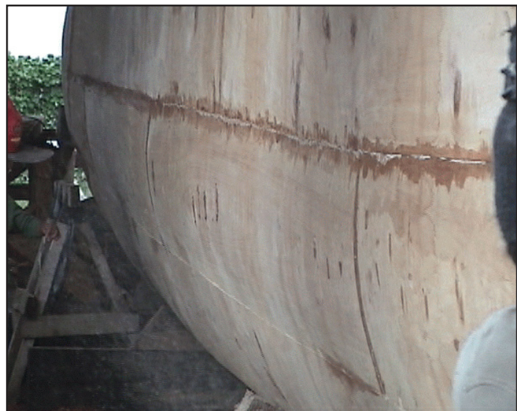
Figure 66. The leeward side of the katea is shown here. Note the relatively straight vertical contour of the hull, with very little tumblehome and an abrupt curvature to the bottom.
