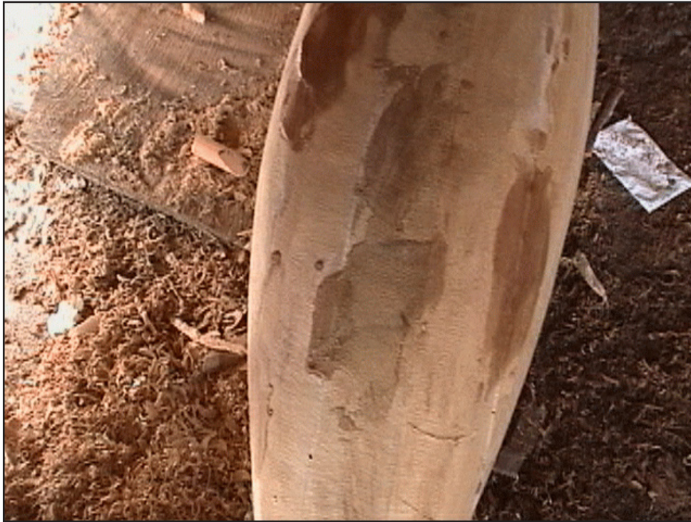
Figure 125. The top of the mast shows the five laminates.
