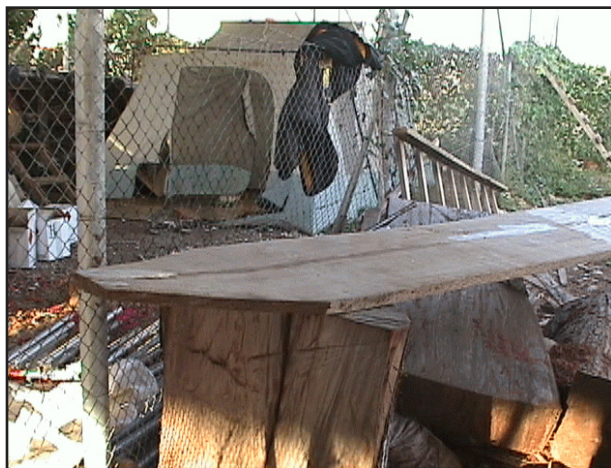
Figure 134. Fohe uli blade. The first 2' from the tip of the paddle blade were tapered until the maximum width of the blade was reached.
