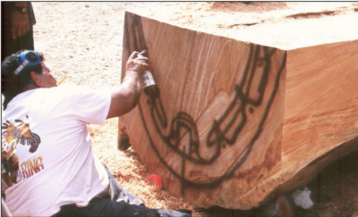
Figure 49. Ribs and their lashings were sketched in.
