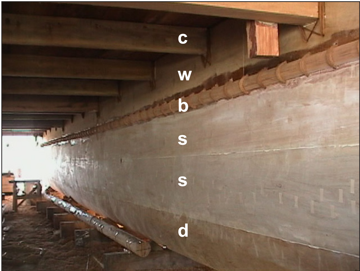
Figure 77. This illustration of the hull shows the multi-layer hull construction with dugout hull segments on the bottom (d), two layers of strakes (s), and the batten (b) which reinforced the joint between the second strake layer and the upper washstrakes (w). There were two planks which made up the washstrake. All twelve crossbooms (c) can be seen running between the two hulls.
