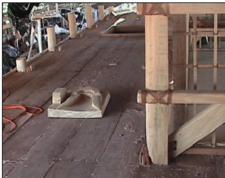
Figure 102. Note the rail posts on the leeward side of the katea and how they rise and fall. This makes it easier to lift the foot of the sail's yard from the rail to the yard groove and back.
