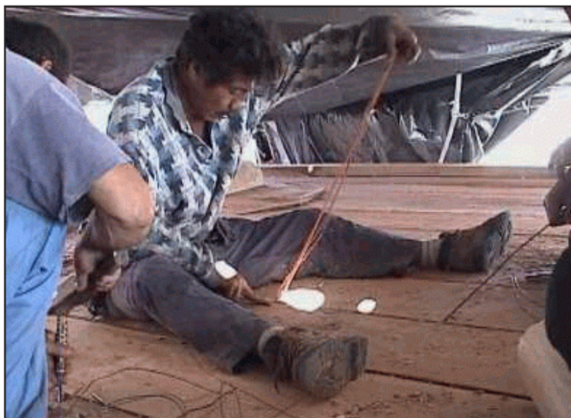
Figure 105. Deck planks ran parallel with the hulls. Here deck planks were being lashed to the crossbooms..
