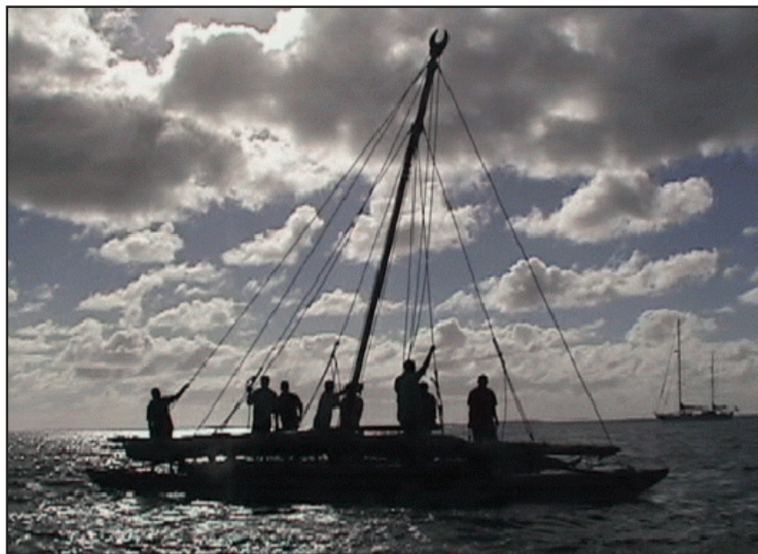
Figure 133. Note the tilt of the mast towards the front prow. In this configuration the foot of the sail yard would be tucked into the right prow and the canoe would be sailing to the right.
