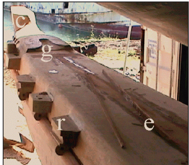
Figure 91. The cutwater (c) is seen at the point of the prow, followed by the yard groove (g). The runners (r) for the mast shrouds are aligned along the left (windward) side. The upper surface of the prow is called the end-cover (e).
