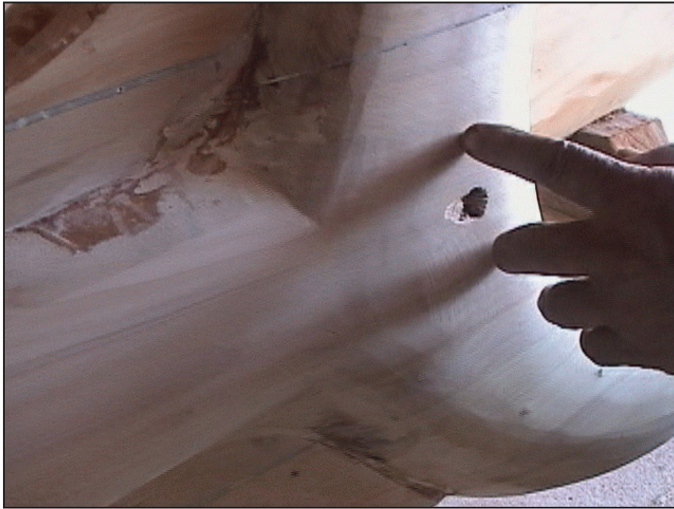
Figure 127. Three holes were to be drilled into the claw for the halyards.
