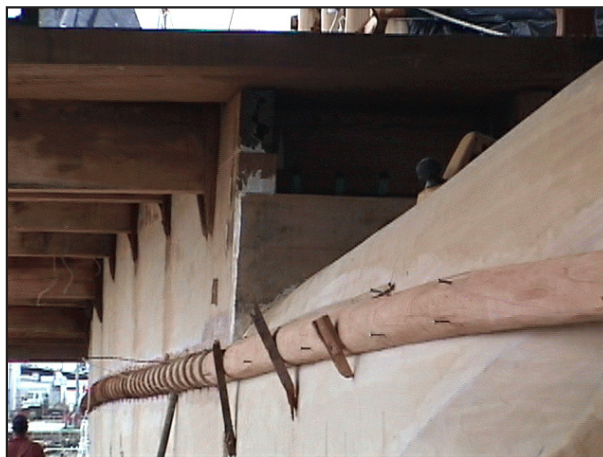
Figure 67. Windward side of the hama is shown here, with a view of the batten, the washstrake above, and the crossbooms.
