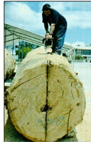
Figure 40. First cut to split log made from top as far down as possible.
