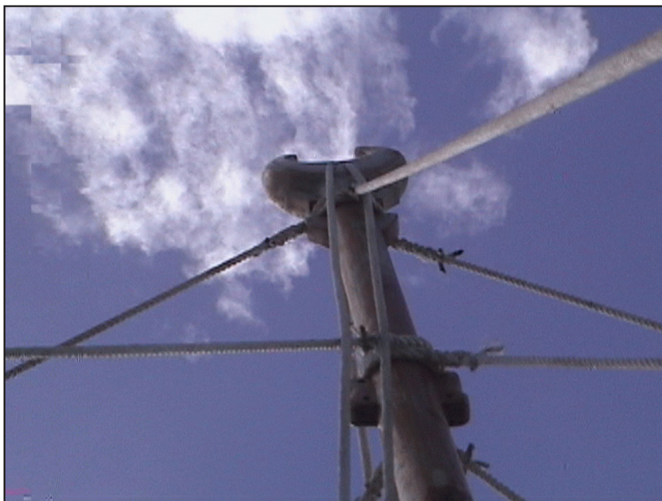
Figure 132. The lower four shrouds just above the two cleats on the mast ran one to each corner of the deck.
