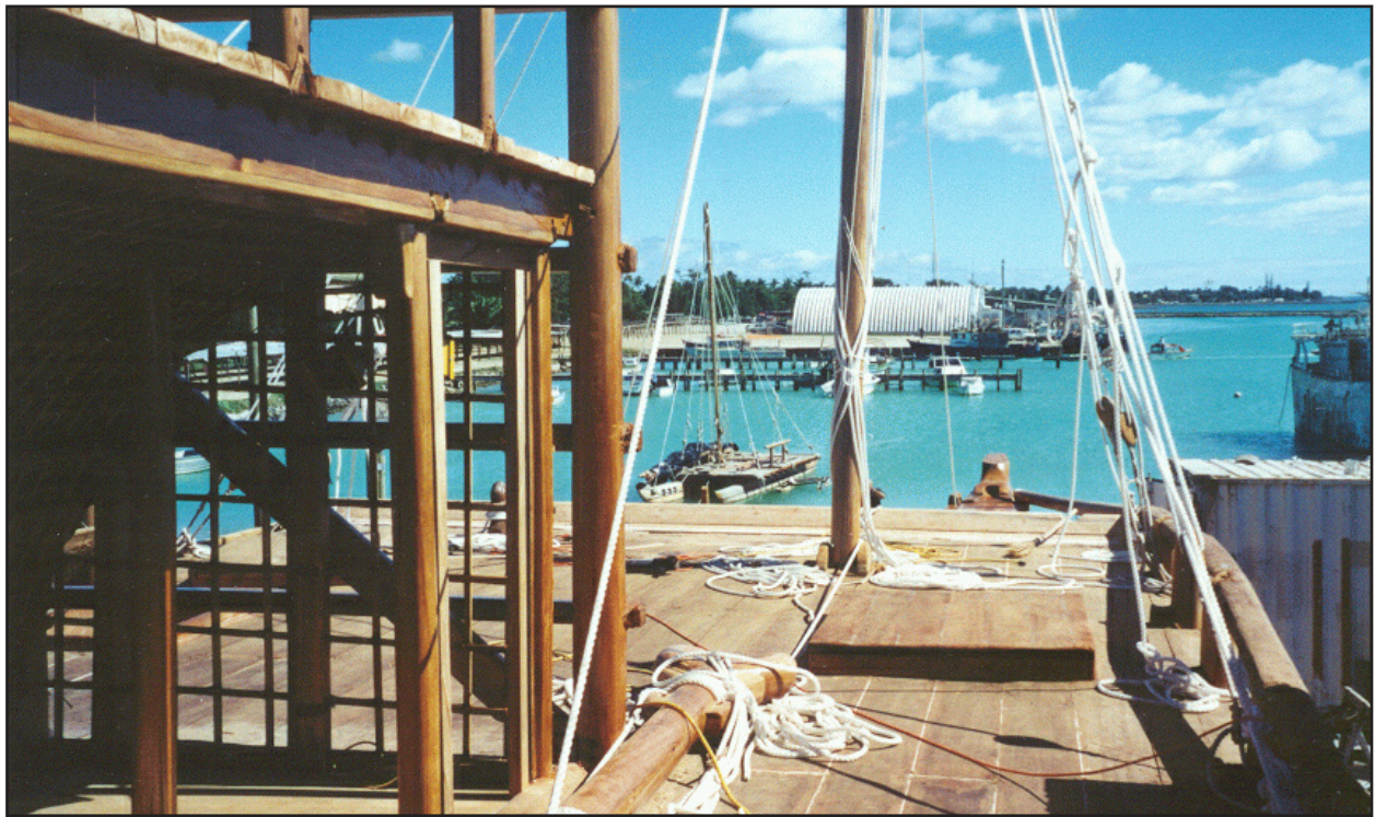
Figure 146. The mast was stepped in place using shrouds and stays. The yard rail can be seen on the right side.
