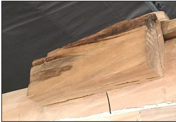
Figure 93. This rotten wood on the end cover was unsuitable for making a runner.
