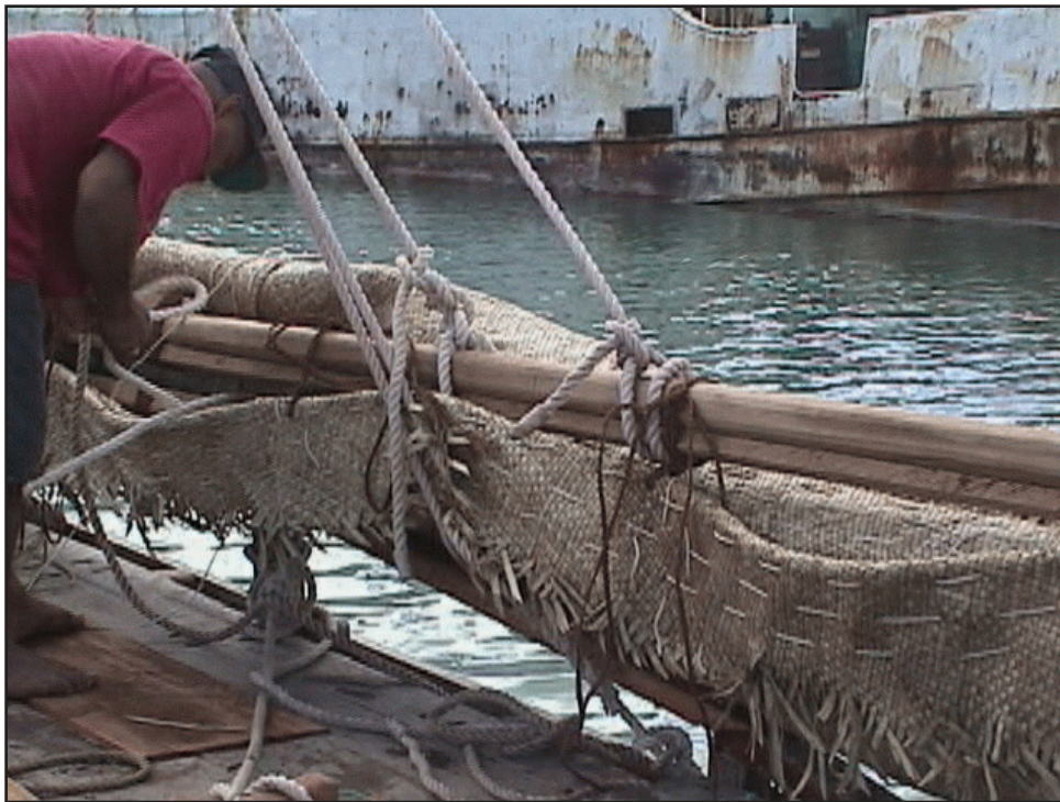
Figure 131. Two halyards were tied on to the sail's yard in preparation for hoisting the sail.
