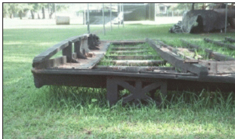
Figure 29. Outrigger and deck of camakau . The * (asterisk) shaped piece is the breakwater. The left side was the yard rail, and leading to the right were the crossbooms which attached to float.
