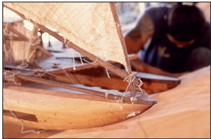
Figure 15. The yard foot is tucked into the groove of the new bow and lashed down.
