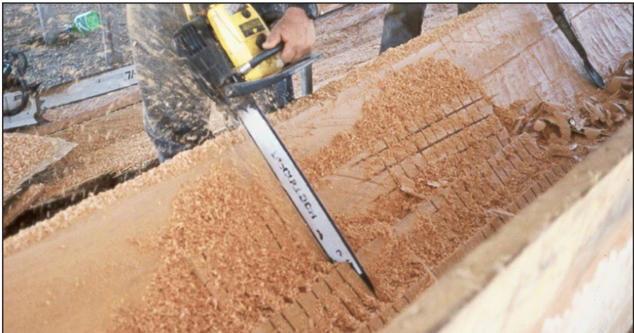
Figure 55. The rest of the hull segment interior was roughed in by crosshatching with a chainsaw and then chipping out the cut sections with a chisel or adze.
