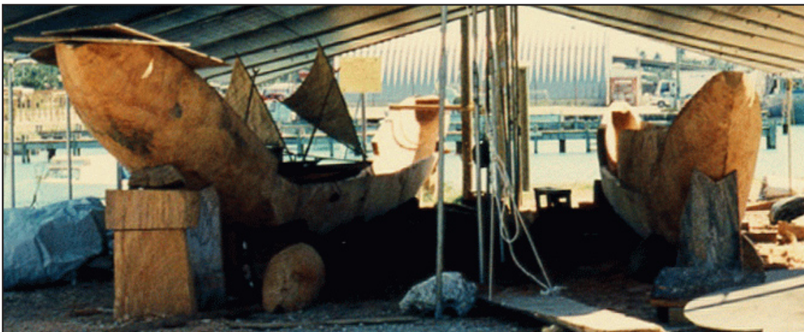
Figure 60. Hull segments laid out in place.
