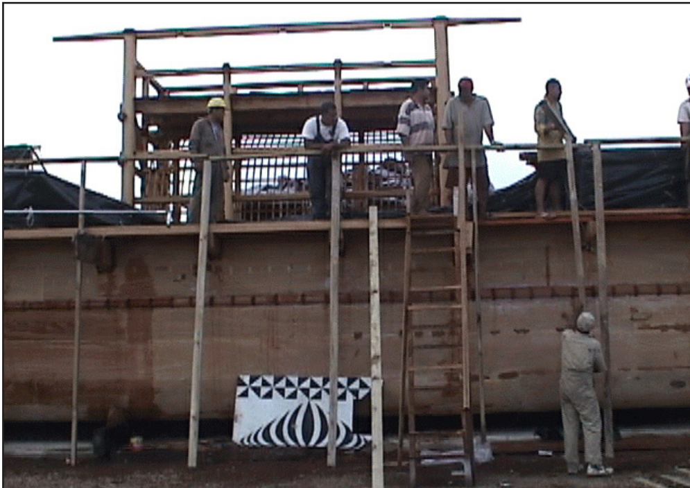
Figure 109. Outrigger hull, fale and lookout deck. From the lookout deck, the captain would stand nearly 15 feet above the water line.
