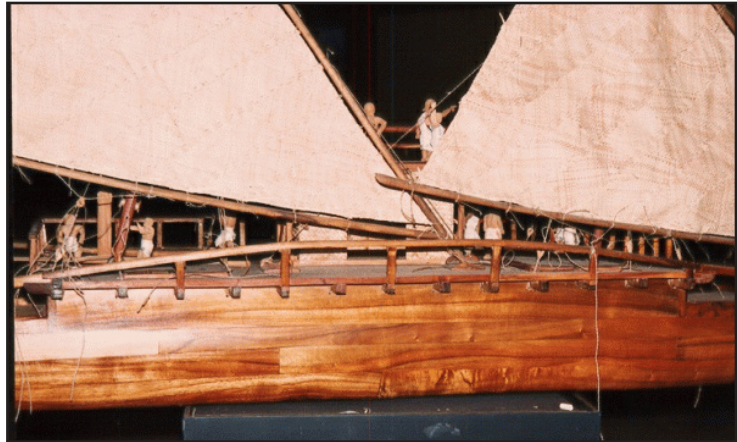
Figure 14. The sail is slid from its previous bow, over the railing, to the “new” bow.
