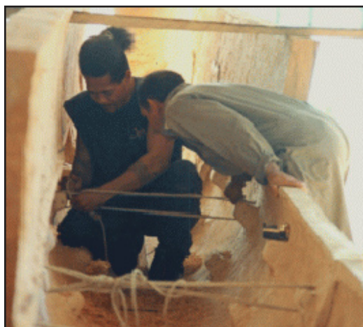
Figure 72. Tourniquet style ropes temporarily reinforced the hull segments.
