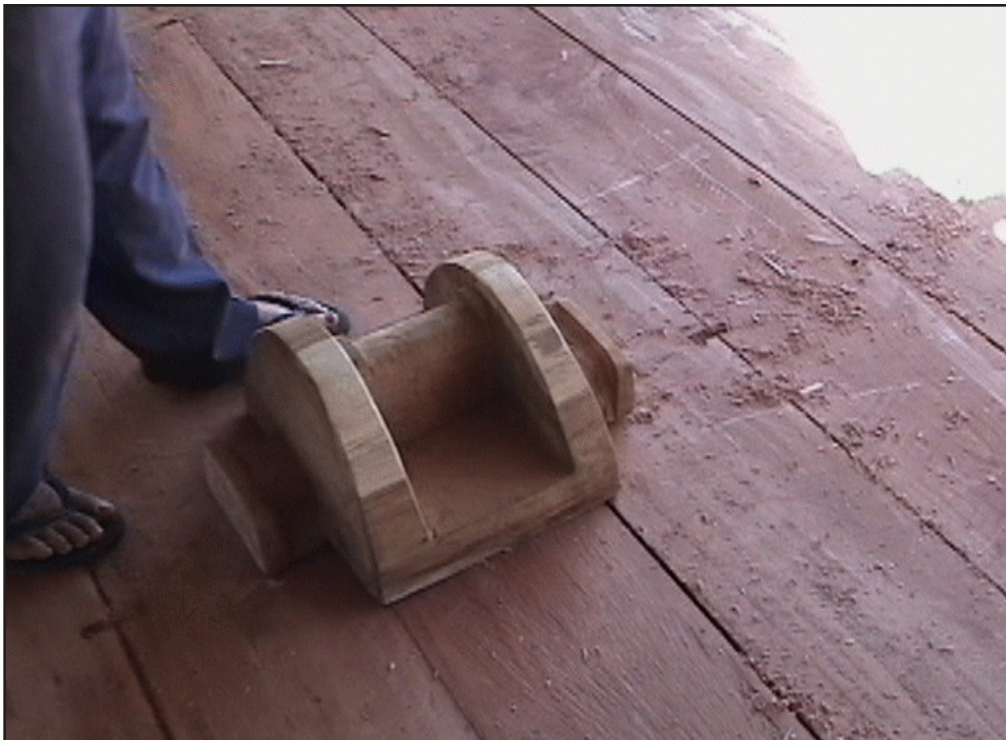
Figure 122. The mast step was placed above a crossboom and lashed by the left and right pieces of the mast step.
