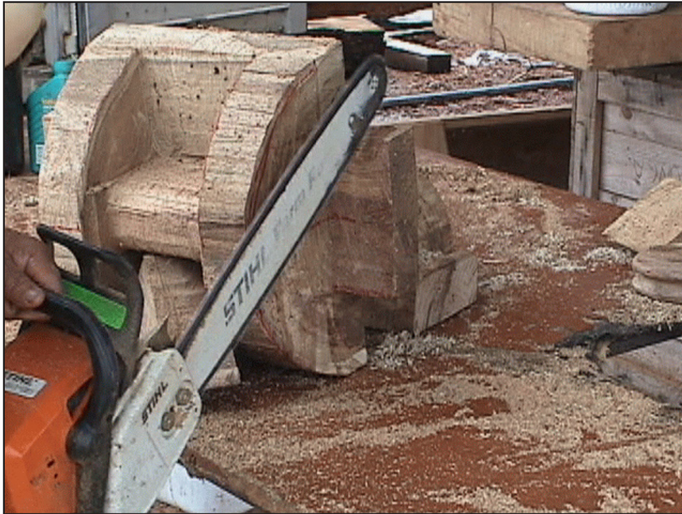
Figure 119. Two side pieces were shaped to provide recessed areas for lashing the mast step down to the deck.
