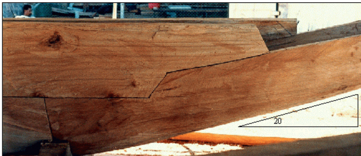
Figure 61. Prow segments were laid at about a 20° angle from horizontal.
