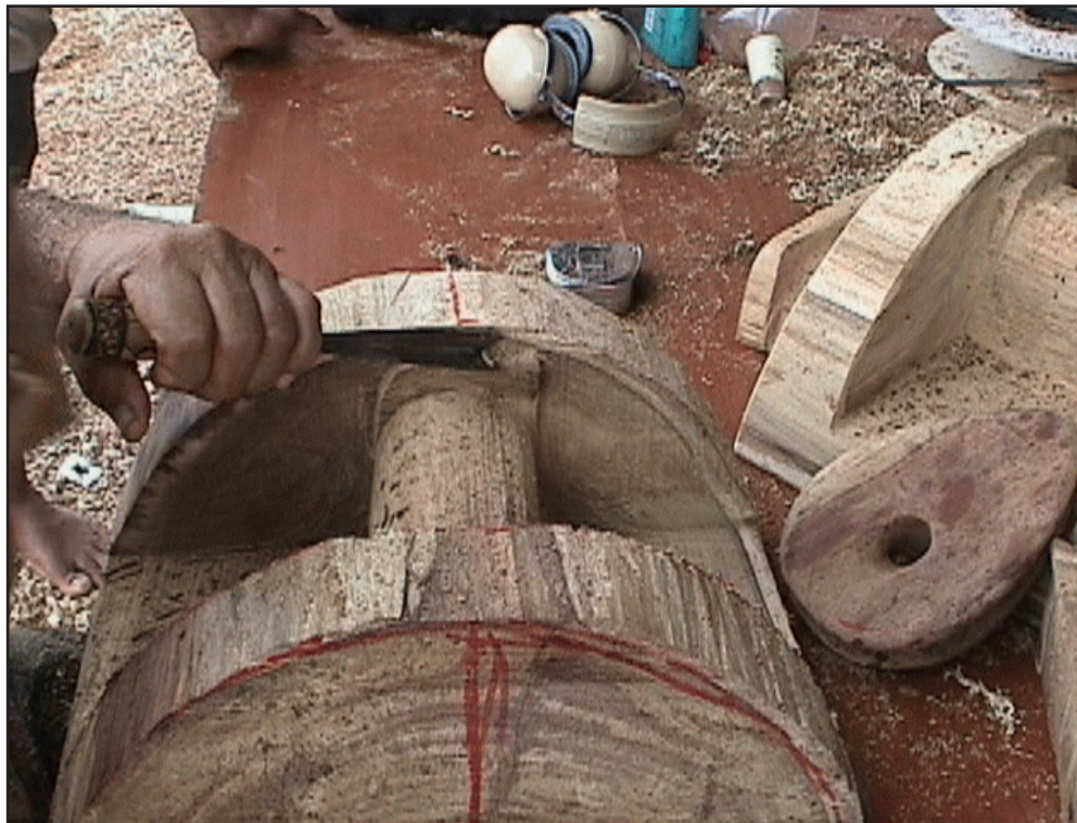
Figure 120. The last detailed trimming was done by hand with a mallet and chisel.
