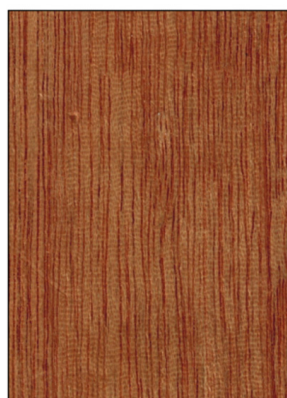
Figure 11. Ripple marks determined by storied rays on a tangential section of Swietenia macrophylla .
