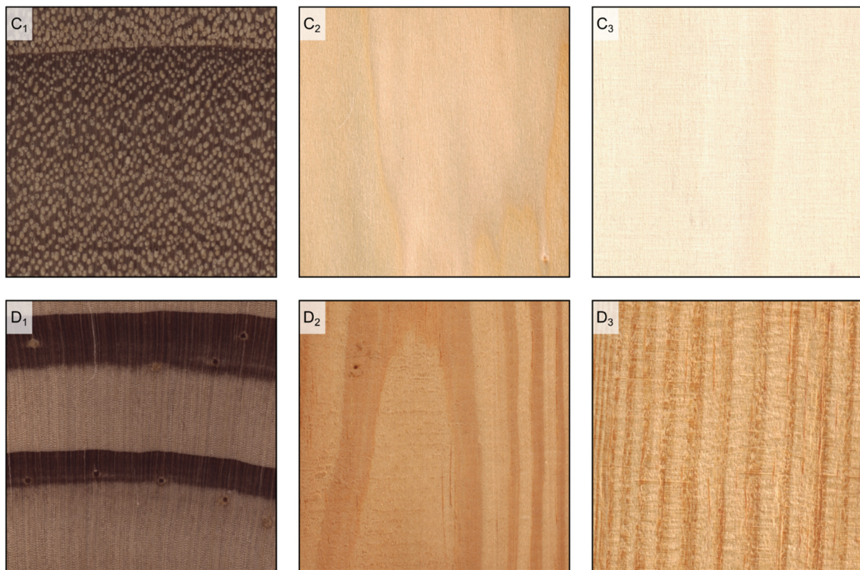
Figure 10. Rays' visibility to the naked eye. In Quercus petraea , some of the rays are clearly more evident than the others on the transverse surface ((A 1 ) transverse section), are visible on the tangential surface and over 5 mm high ((A 2 ) longitudinal tangential surface), and visible on the radial surface ((A 3 ) longitudinal radial surface); in Platanus occidentalis , rays are visible on the transverse surface and noded ((B 1 ) transverse section), they are visible on the tangential surface and less than 5 mm high ((B 2 ) longitudinal tangential surface), and visible on the radial surface ((B 3 ) longitudinal radial surface); in Populus tremula , rays are not visible on either the transverse surface ((C 1 ) transverse section) and the tangential surface ((C 2 ) longitudinal tangential surface), while barely noticeable on the radial surface ((C 3 ) longitudinal radial surface); in Pinus sylvestris , rays are not visible on either the transverse surface ((D 1 ) transverse section) and the tangential surface ((D 2 ) tangential surface), while barely noticeable on the radial surface ((D 3 ) longitudinal radial surface).
