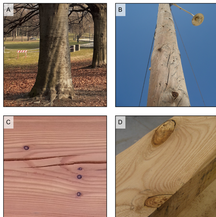
Figure 15. (A) spiral grain is visible in the tree in the foreground, while it is not present in that in the background ( Fagus sp.); (B) spiral grain in a softwood pole. Grain deviates around knots ((C) small knots on Larix decidua ; (D) pair of knots on Castanea sativa ).
