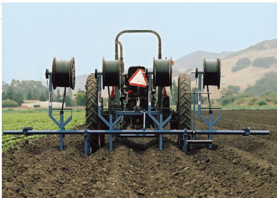
Specialized equipment (shown here, by Andros Engineering) is used to install drip tape 8 to 12 inches below the soil surface, at a cost of about $600 to $1,000 per acre. Despite this price, studies show that improved irrigation efficiency and yield benefits increase profits for growers in the San Joaquin Valley, compared with sprinkle or furrow irrigation.
