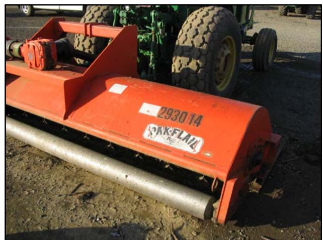
Figure 22. Flail mower (Photo: Guy Kyser)
