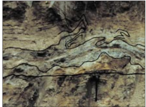
Figure 3. Photograph and interpreted line drawing of overturned and detached folds in the Scotts Corners Formation (Qsc) at site a. Original land surface is located approximately 1.5 ft above the frame. Tc—Calvert Formation.
