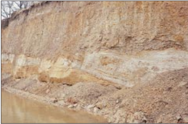
Figure 20. Photograph of a channel (light gray) at the base of the upper mud. Channel cuts into cross-bedded sand below. Approximately 20-ft exposure located along south wall.
