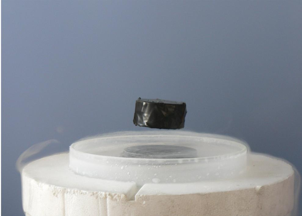
Cooper pairs are charged, and respond to magnetism in a curious way: their motion modifies to eject magnetic field from the superconductor. This enables magnets to levitate on superconductors, and is used in some Maglev trains.
