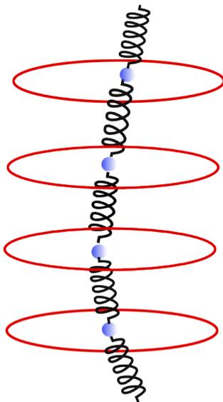
Each ball is constrained to move on a disc. The coordinate of each ball on its disc represents the field components  $\phi_1$  and  $\phi_2$  for that position along the chain.
