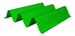
The field remains constant as we move perpendicular to the direction of propagation. So, we can always just consider the wave equation with one space direction, x, which is parallel to the direction of propagation. The field is constant when moving perpendicular to the direction of propagation.
