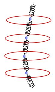
Each ball is constrained to move on a disc. The coordinate of each ball on its disc represents the field components  $\phi_1$  and  $\phi_2$  for that position along the chain.
