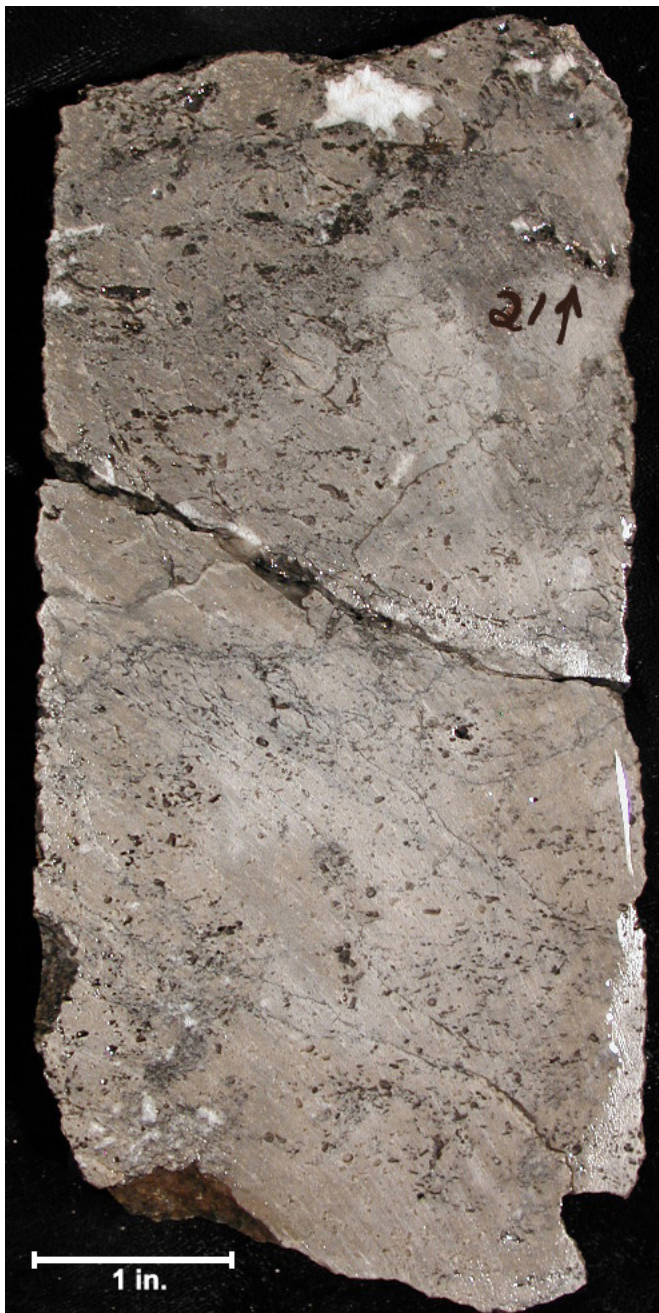
Figure 3.7. Typical peloidal/skeletal packstone/wackestone representing moderate-energy, open-marine, shoal-flank lithofacies. Lisbon No. B-816 (NE1/4SW1/4 section 16, T. 30 S., R. 24 E., SLBL&M [figure 2.3]); slabbed core from 8521 feet (2597 m).
