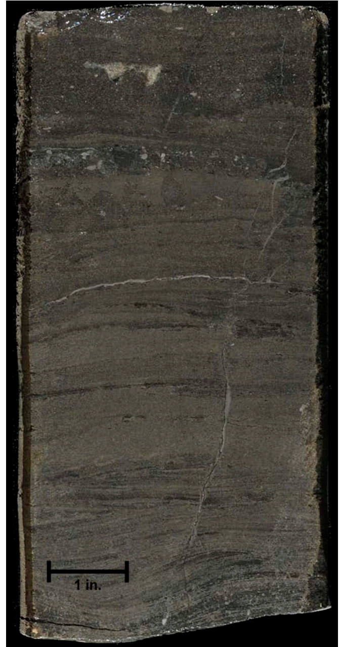
Figure 5.8. Cores displaying Leadville open marine facies. (A) Crinoidal/skeletal packstone to grainstone representing a shallow crinoidal shoal; Salt Wash No. 1 Floy well, 9469 feet (2886 m), Salt Wash field (figure 5.2). (B) Porous algal (microbial) boundstone to mudstone representing a possible Waulsortian mound; No. 1 Big Indian well, 10,081 feet (3073 m), Big Indian field (figure 5.2).
