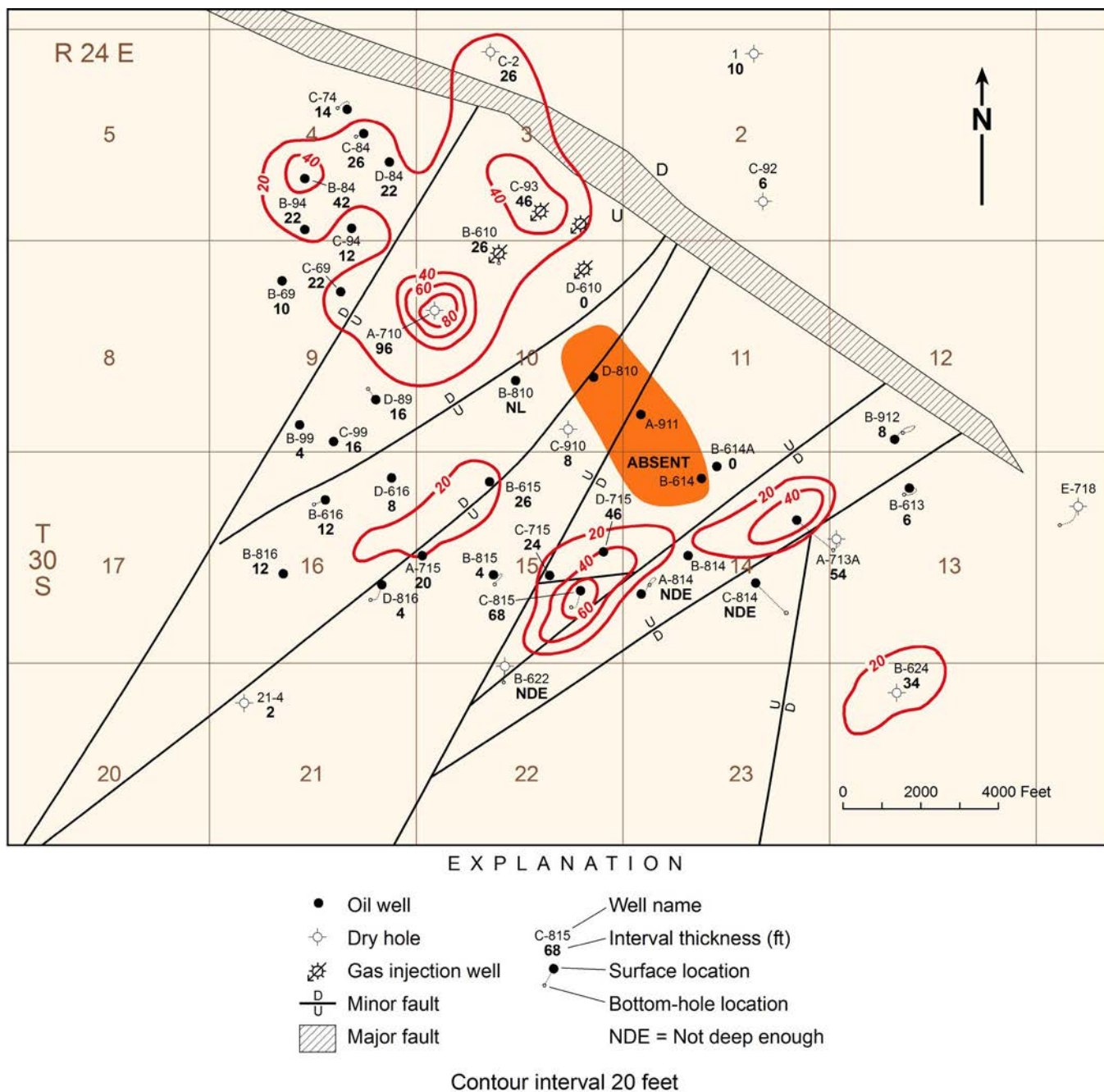
Figure 2.10. Net feet of porosity isochore for reservoir zone 1, Leadville Limestone, Lisbon field.
