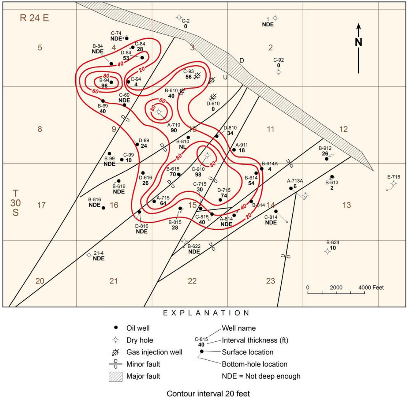
Figure 2.12. Net feet of porosity isochore for reservoir zone 3, Leadville Limestone, Lisbon field.
