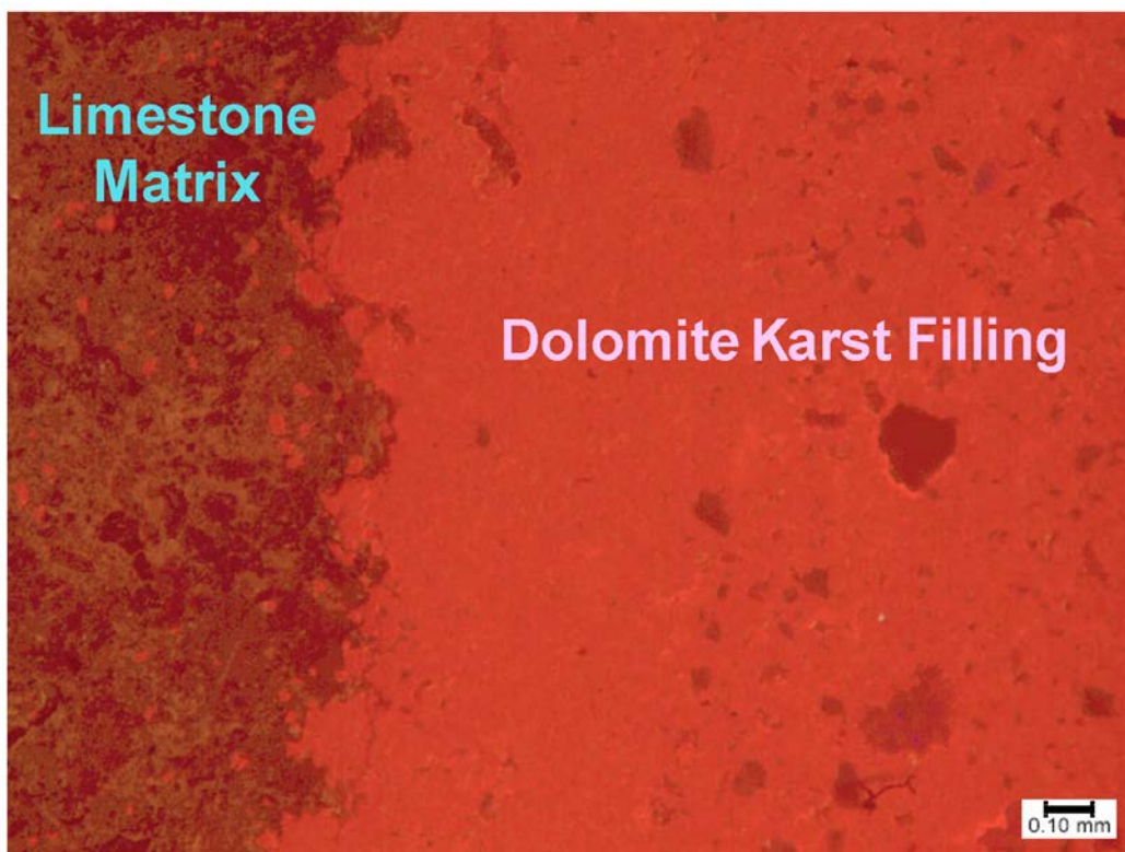
Figure 4.36. Photomicrograph from Lisbon No. D-616 well at 8308 feet (2532 m). This low-magnification image nicely shows a sharp contact that runs from top to bottom toward the left side of the photomicrograph. The bright red field is composed mostly of dolomite, whereas the field with the orangish cast (to the left) is almost entirely limestone. The dolomite area is composed of carbonate grains and sediments that have filled a karst-related crack or cavity. The poorly sorted, angular grains that are “floating” within the dolomite field are a combination of detrital siliciclastic (mostly quartz) grains and lithified limestone clasts. The limestone field along the left side of the photomicrograph is composed of non-luminescent skeletal (crinoid-rich) sediments with orangish cements. Neither the dolomite with siliclastic sediments nor the limestone display any visible matrix porosity. The contact between the dolomite and limestone fields is irregular but sharp. Finally, few scattered replacement dolomite rhombs (also with red luminescence) are within the well-cemented limestone. Figure 4.9C is the same field of view under crossed nicols.
