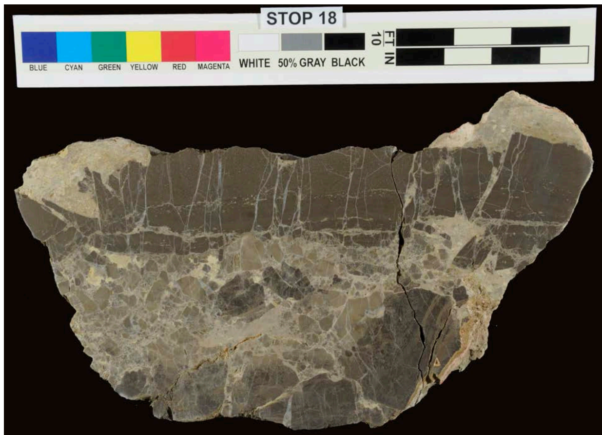
Figure 10.20. Slabbed specimen of highly brecciated rock typical of that present at study site 3.
