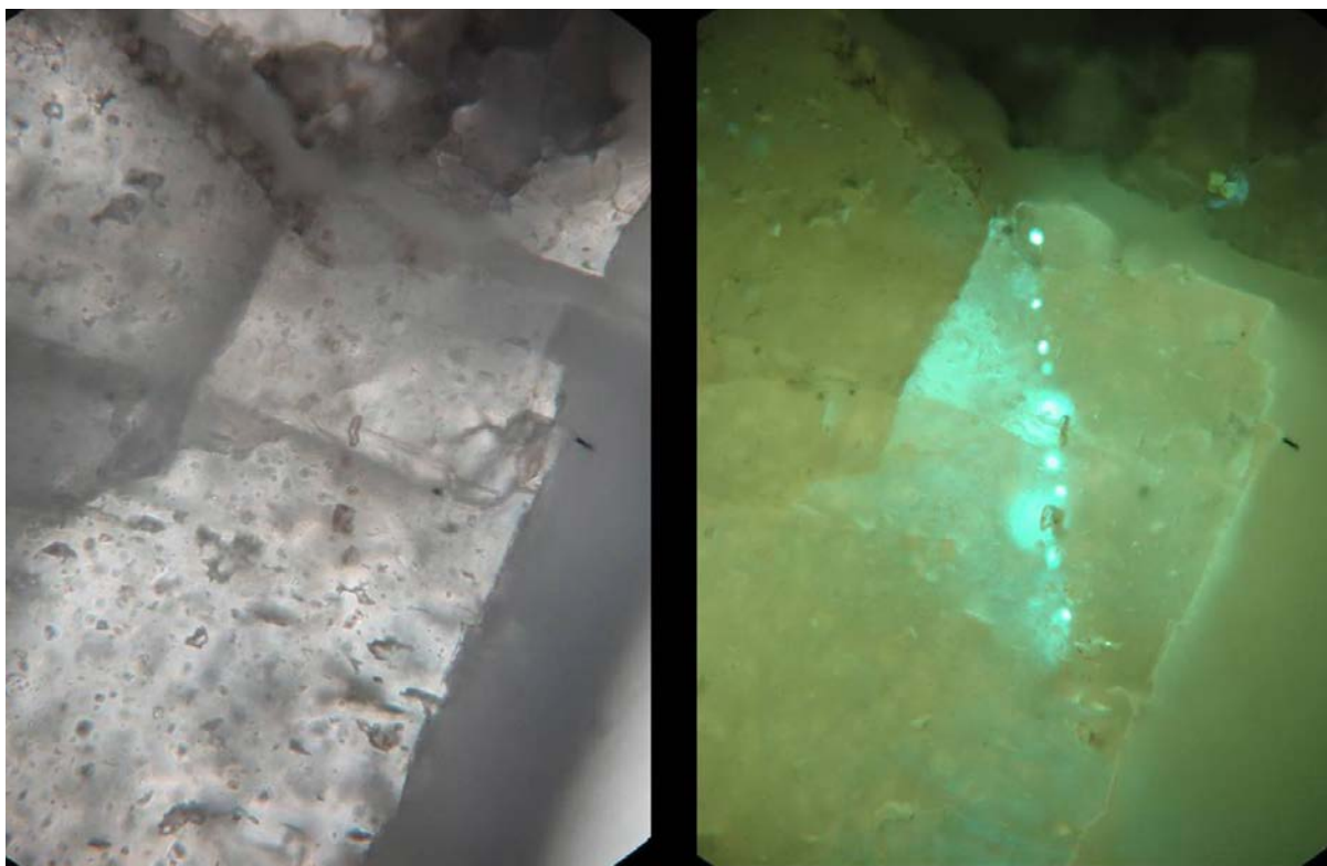
Figure 4.60. Secondary oil inclusions in calcite from the Lisbon No. D-616 well at 8372 feet (2552 m). The height of each image is 0.3 mm. Right-hand image was taken under fluorescent light.
