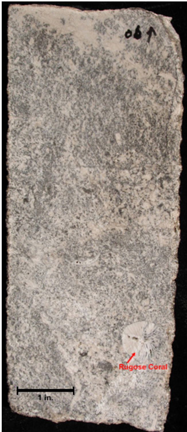
Figure 3.5. Typical crinoidal/skeletal grainstone/packstones representing high-energy, open-marine shoal lithofacies, Lisbon No. B-816 (NE1/4SW1/4 section 16, T. 30 S., R. 24 E., SLBL&M [figure 2.3]). (A) Slabbed core from 8506.5 feet (2592.8 m). Note the large rugose coral. (B) Slabbed core from 8547 feet (2605 m).
