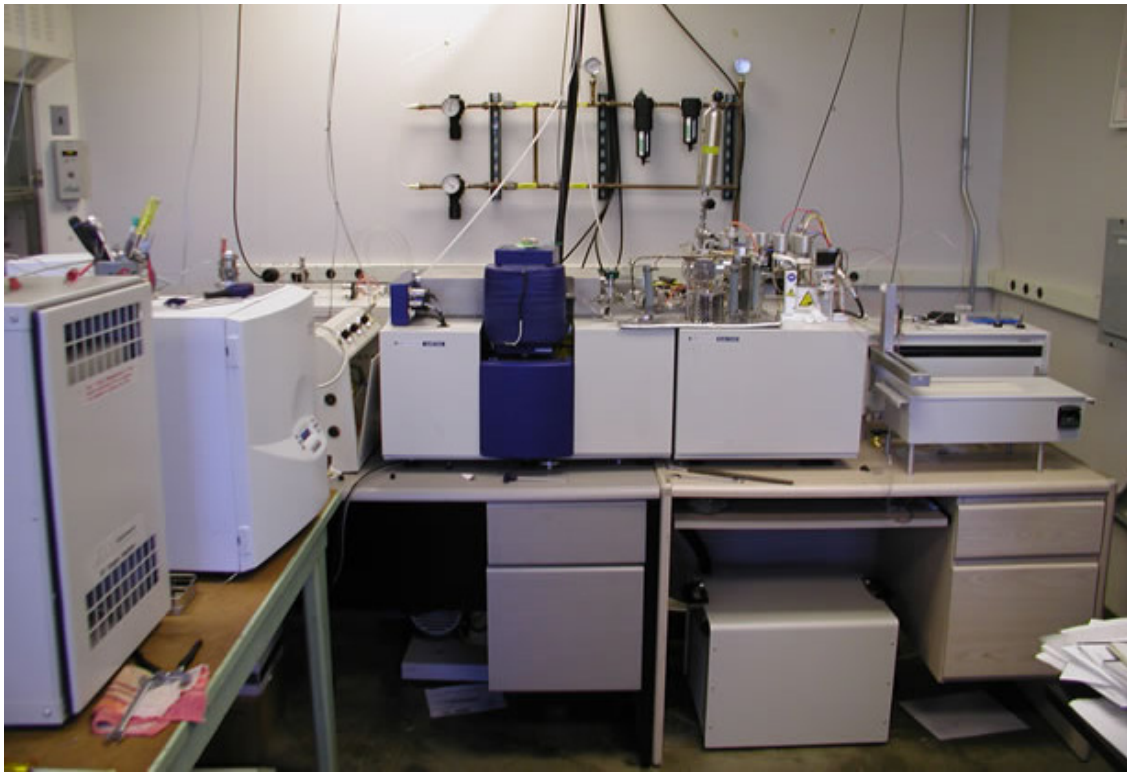
Figure 4.64. The Colorado School of Mines Stable Isotope Laboratory's GV Instruments IsoPrime stable isotope ratio mass spectrometer. Several peripheral devices are interfaced with the IsoPrime for both dual-inlet and continuous flow applications.
