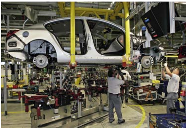
LIFTED: Opel mechanics assembling an Insignia in Rüsselsheim.
