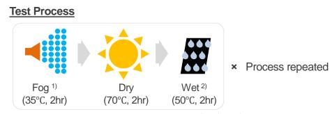
Test process is conducted according to ISO 14933.
