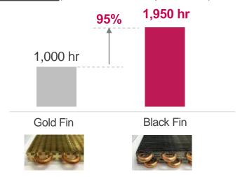
CCT (Cyclic Corrosion Test)
