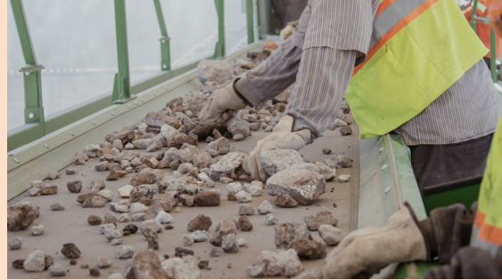
C&DW processing belt at a recycling plant, México.
