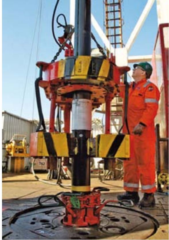
■ Supervising the fastening of the VAM® connections is the daily mission of VAM Field Service technicians.
