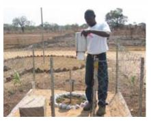
Under the flood-warning system, precipitation levels are measured daily and critical readings reported.
