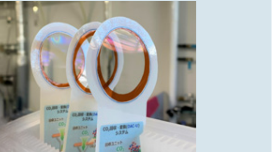
Membrane with a width of 1/300 of a strand of human hair
