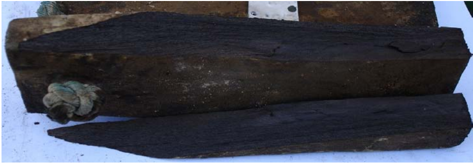
Figure 10: Treated samples of Keruing after 168 months exposing in seawater
