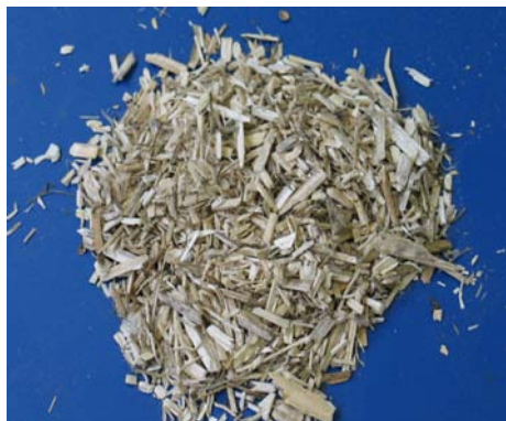
Figure 4: Hemp shives, middle layer material (ML)
