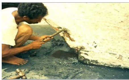
Figure 2: Removing lime and lipid combination from Hull planking
