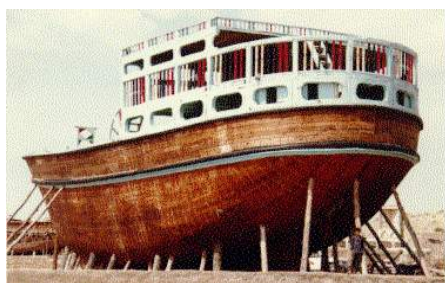
Figure 1: Hull planking of wooden vessel by Teak wood
