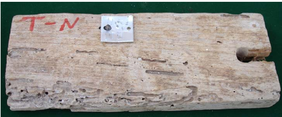
Figure 4: Heavy attack of untreated Teak sample
