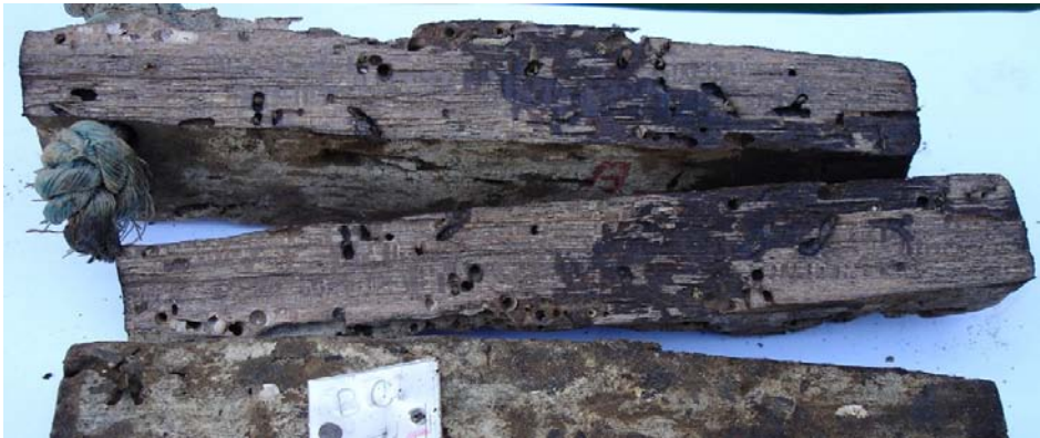
Figure 8: Treated samples of Balau after 168 months exposing in seawater
