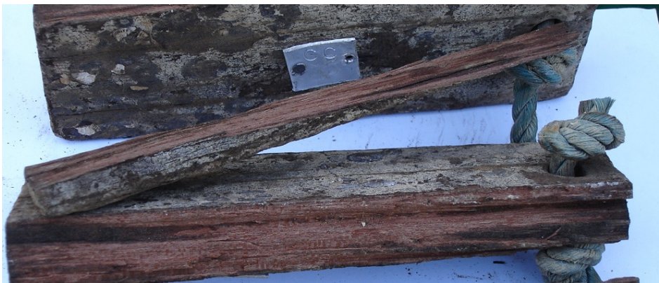
Figure 9: Treated samples of Chengal after 168 months exposing in seawater
