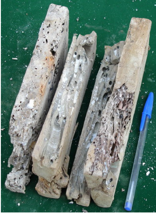
Figure 8: Samples of Oak, Hornbeam and Beech treated by Celcure
