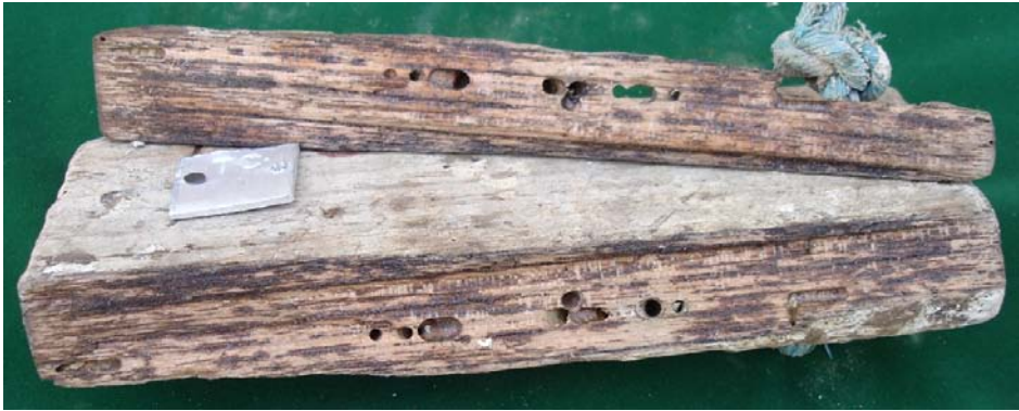
Figure 7: Treated samples of Teak after 168 months exposing in seawater
