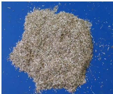
Figure 5: Hemp shives and leaves, surface layer material (SL)
