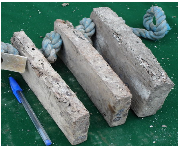
Figure 9: Samples of Oak, Hornbeam and Beech treated by Creosote
