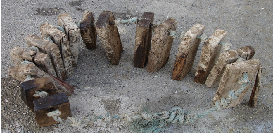
Figure 3: Treated samples' frame was removed from the seawater and carefully scraped
