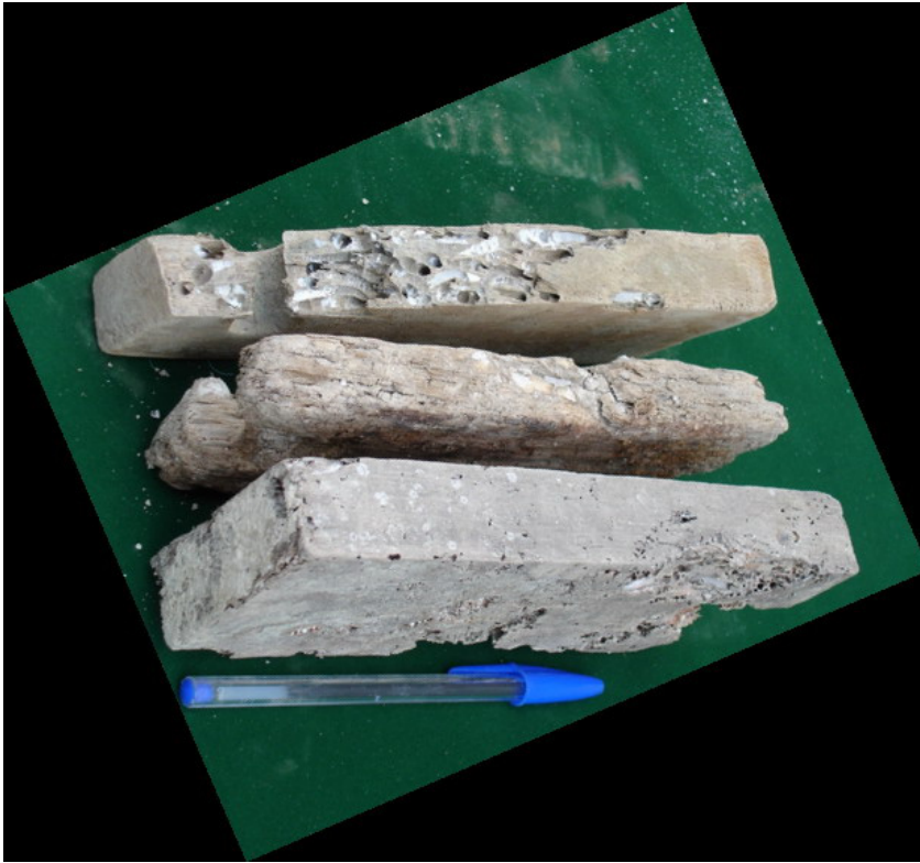
Figure 6: Samples of Oak, Hornbeam and Beech treated by Creosote
