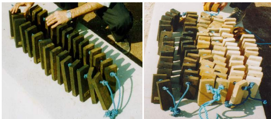
Figure 2: Making space by tying the rope between the samples
