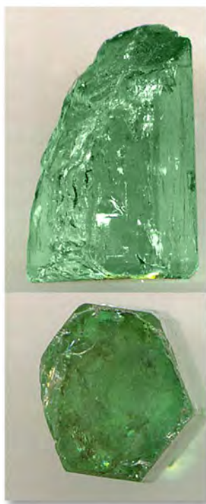
Fig 7.4.16 – Flux-grown (melt) synthetic emeralds have no water in their crystal matrix, whereas all natural emeralds do. Natural emeralds grow in the same manner as quartz but higher pressures and temperatures.
