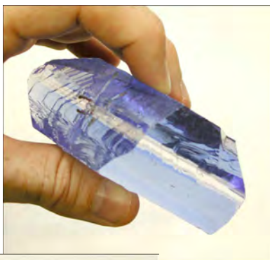
Fig 7.4.14 – This is a man-made quartz crystal grown for technological purposes. The clear strip seen in the bottom photo is the quartz ‘seed’ while the blue material is the grown quartz. The addition of the element chromium is responsible for the blue color.
