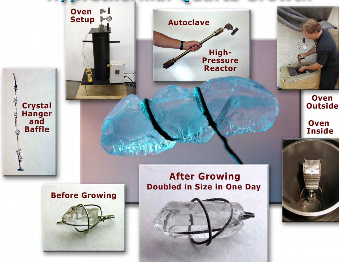
Fig 7.4.13 – This diagram illustrates the hyprethermal quartz-growth process. The word hyprethermal is a merger of the words “hydro” (water), “pre” (pressure), and “thermal” (heat). A combination of these three physical properties creates a pressurized thermal environment in which quartz crystals can grow. In this diagram, a hanger holding quartz crystal seeds is placed in the high-pressure reactor. A water solution is added to the reactor and it is placed in an oven and heated until the solution reaches 350-400° C. Compare the images of the crystal before growing and after growing. The crystals experienced a rapid growth rate approximately doubling in size in one day , not over millions or even thousands of years.
