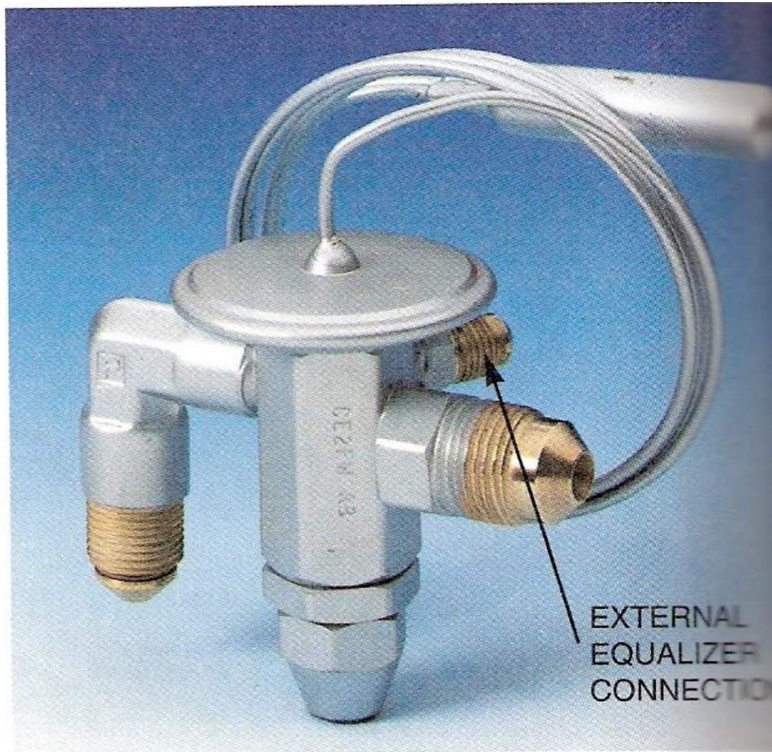
Figure 24–10 The third connection on this expansion valve is called the external equalizer. Courtesy Parker Hannifin Corp.
