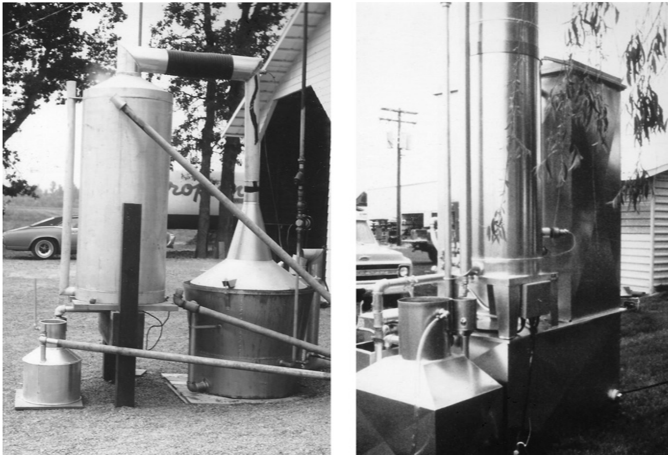
FIGURE 6.5 Two examples of distillate water redistillation systems. The one on the left designed by Cobb manufacturing and the one on the right by Newhouse Manufacturing, Inc.
