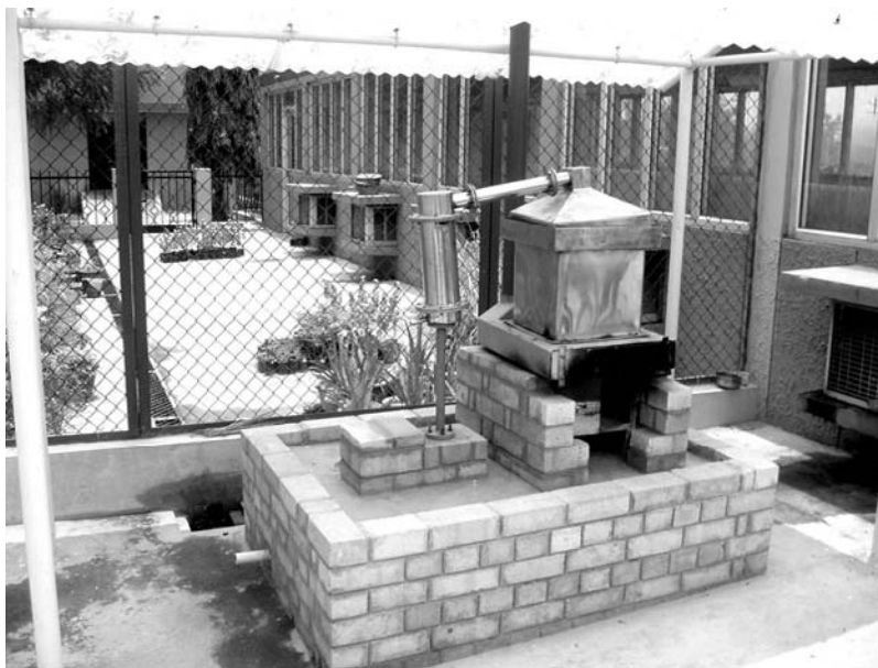
FIGURE 6.7 Newly designed field still by CIMAP.
