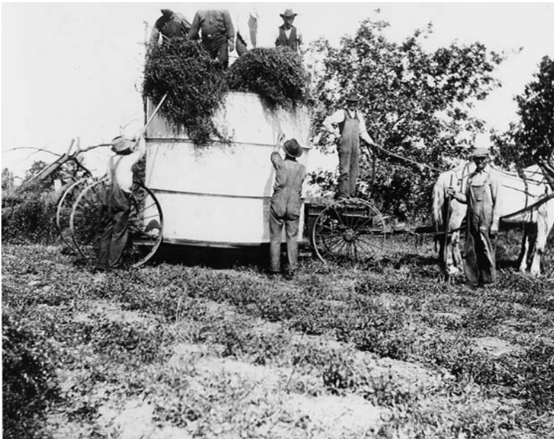
FIGURE 6.4 Examples of the tub (trailer still) designs that have been used in the United States over the years.
