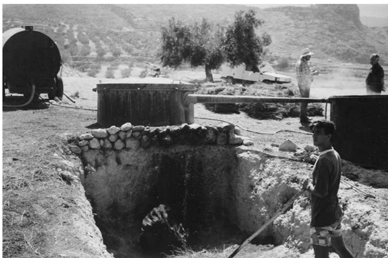
FIGURE 6.1 Typical direct-fired field still used for production of pennyroyal oil in Spain.
