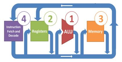
• The datapath elements are the functional blocks within a microprocessor that actually interact to perform computational operations. These tasks include reading/writing to memory, arithmetic, logic operations, and numerical shift operations
