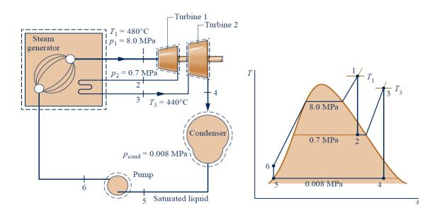
To begin, we fix each of the principal states. Starting at the inlet to the first turbine stage, the pressure is 8.0 MPa and the temperature is 480oC, so the steam is a superheated vapor. h1=3348.4 kJ/kg and s1=6.6586 kJ/kg .K.
