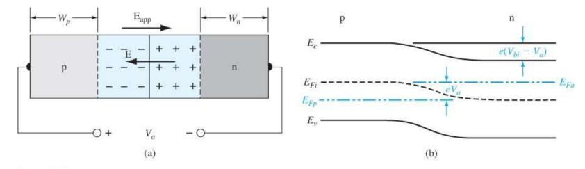
**Figure 8.3** (a) A pn junction with an applied forward-bias voltage showing the directions of the electric field induced by  $V_a$  and the space charge electric field. (b) Energy-band diagram of the forward-biased pn junction.
