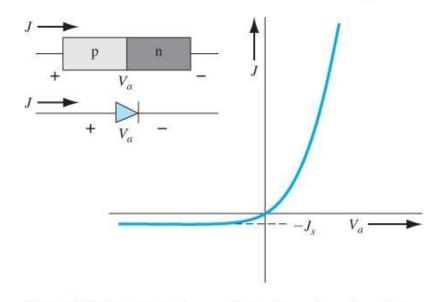
If the voltage Va becomes negative (reverse bias) by a few kT eV, then the reverse-biased current density becomes independent of the reverse-biased voltage. The parameter Js is then referred to as **the reverse-saturation** current density.
