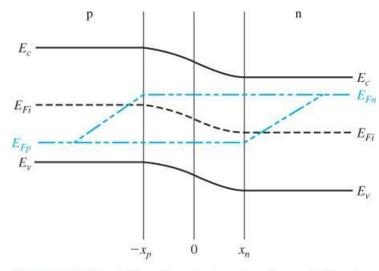
Figure 8.5 | Steady-state minority carrier concentrations in a pn junction under forward bias.
