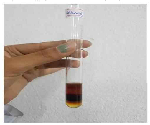
**Caution:** In order for this test to be successful, the tubes must be dry and the solutions should be non-aqueous.
