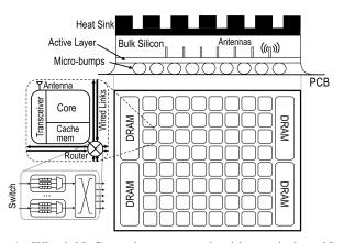
Fig. 1: Wired NoC mesh augmented with a wireless NoC within a conventional flip-chip package with one vertical monopole antenna and transceiver per core.
