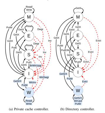
Fig. 4: Transitions between stable states of *WiDir* in the controllers of the private cache (a), and directory (b). In the figures, black lines are core-initiated transactions; dashed red lines are directory-initiated transactions; and the blue text is the added wireless coherence transitions.
