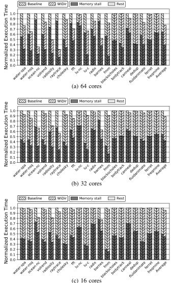
Fig. 8: Execution time in *WiDir* and *Baseline*, normalized to *Baseline* for 64 (a), 32 (b), and 16 (c) core executions. The bars are broken down into memory stall cycles and the rest of cycles.
