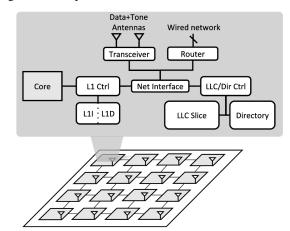
Fig. 2: Manycore that supports the WiDir protocol.
