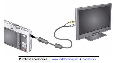
NOTE: Ensure that the Video Out setting (NTSC or PAL) is correct (see page 31). The slide show stops if you connect or disconnect the cable while the slide show is running. (Image quality on a television screen may not be as good as on a computer monitor or when printed.)
