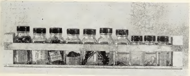
Fig. 3, Tray with removable center strip taken out to permit storage of two sizes of square bottles containing large specimens.
