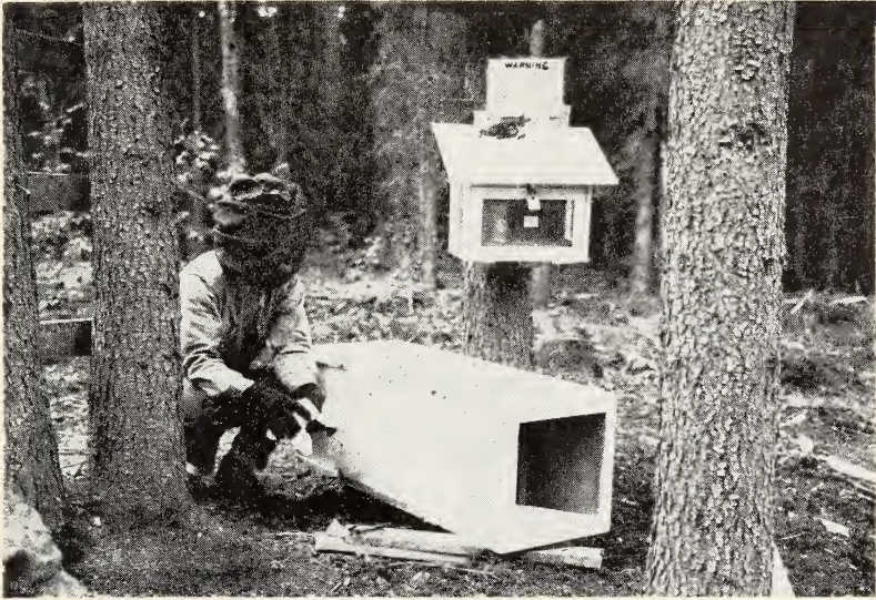
Fig. 3.—Weather box and bait box at ground level of the tower shown in Fig. 2. The weather box housed a hygrothermograph.
