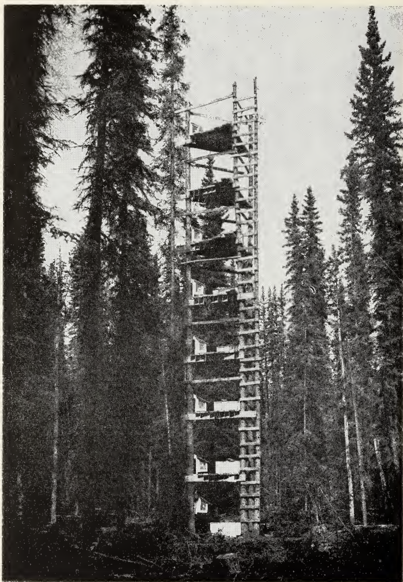
Fig. 2.—Tower constructed in Nordale Woods to study the vertical distribution of mosquitoes in a forested area. Weather boxes with hygrothermographs and "bait boxes" used in studying host attraction of subarctic mosquitoes were placed on the ground and at each level. Highest level was 42 feet above the ground.
