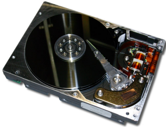
Figure 3 A partially dismantled hard drive, showing the disc inside.
