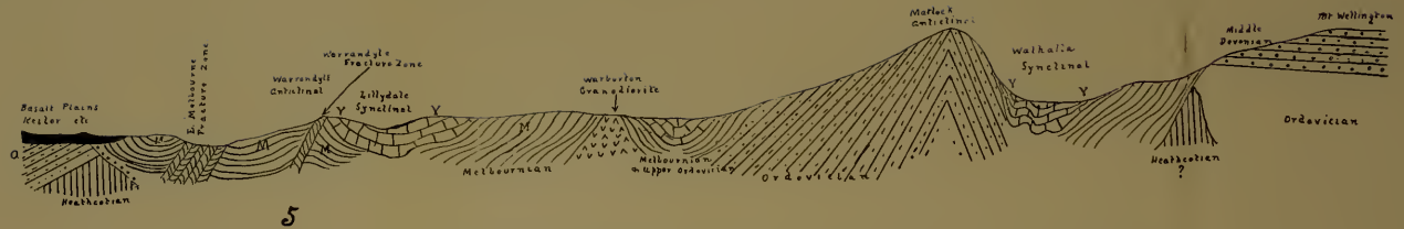
Diagrammatic Section from West of Melbourne along the Yarra to across the Macallister River to Mt Wellington, showing the chief folds and fracture Zones of the Silurian System, the relations of the Yeringian and Melbourneian series, and the probable occurrence of Heathcotean rocks on both sides of the Silurian basin.
