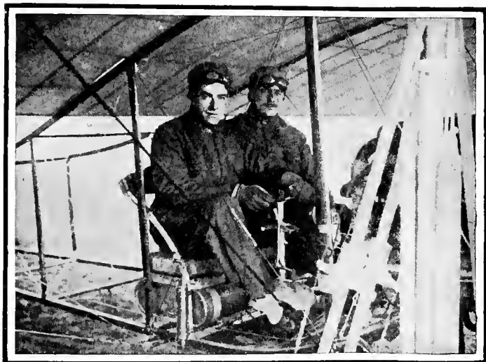
Grahame-White on his Bleriot No. XI. The lever in front of him operates all the controls through the movement of the drum at its base.
