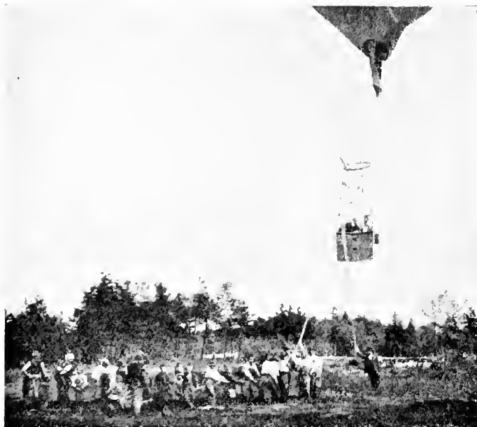
Making a landing with the aid of bystanders to pull down upon the trail-rope and a holding rope.
