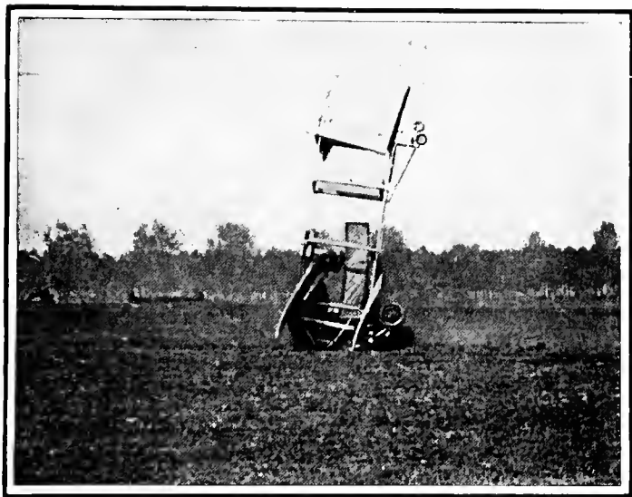
Result of a failure to deflect the planes quickly enough when the engine stopped. The operator fortunately escaped with but a few bruises.
