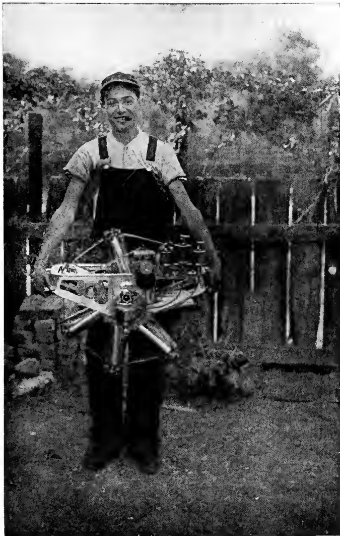
The Holmes rotative engine, 7-cylinder 35 horse-power, weighing 160 pounds. An American engine built in Chicago, Ill.
