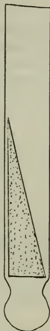
FIG. 211.—Culture tube with bulb to hold glycerine and water below slant of vegetable.
