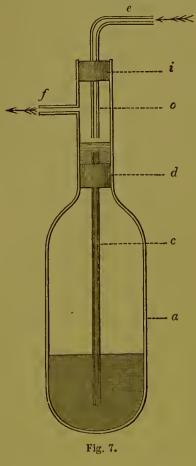
tube c, which passes through the perforated  $\operatorname{cork} d$ , and flows into the space above this cork. The tube e is connected by a piece of rubber tubing with a gas-jet, and the gas continues to pass through the tube f to the Bunsen burner, unless arrested by the rising of the mercury, which acts as a valve to close the lower extremity of the tube e. This tube is adjustable through the cork i, and it is evident that the temperature at which the gas supply is shut off
