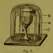
a, wine-glass; b, glass cover (watch-glass); c, bell-glass, supported by a square glass plate. ination by atmospheric germs. The culture-flasks employed contain from one to four fluid drachms. "They are made from glass-tubing of three or four tenths inch diameter, and those which the writer has used in his numerous experiments have all been homemade. It is easier to make
