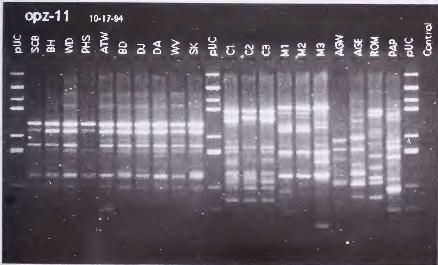
Figure 2. Photo of gel produced using RAPD amplification of total genomic DNA with primer OPZ-11.
