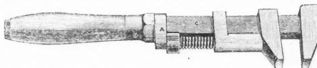
All consumers have noticed that their wrenches first fail by reason of the force exerted on the handle, and by the springing of the bar. Our improvement provides both these defects, the jaws being flushed wider than any other wrench in market, and the handle cannot be displaced, as all strain on it is taken by the screw threads; D. (see cut). Already adopted as the best by the principal railroads and machine shops, and for sale by Hardware Dealers generally.
