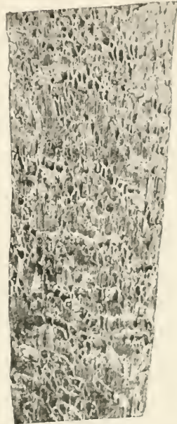
FIG. 261. — Stereum trivestitum . Later stages of Oak-wood destruction. Longitudinal section showing holes in the timber. (v. Tubelf phot.)
