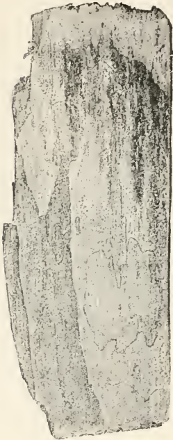
FIG. 279.— Polyporus Hartigii . Destruction of wood of Silver Fir. The decayed wood is yellow, but shows dark points and black lines. (v. Tubeuf phot.)
