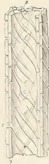
FIG. 280.—Tracheid of Pinus destroyed by Polyporus stipitoides . The cellulose has been for the most part extracted, and the walls consist of lignin (wood-gum). Cracks occur in the dry secondary wall, while the wall ( a, b ) remains intact. The spiral structure of the secondary wall causes crossing of the fissures in the walls of adjoining cells at the bordered pits, c , and at bore-holes, d, e ; where neither pits nor holes are present the fissures are simple, f . (After R. Hartig.)
