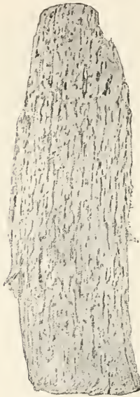
FIG. 273.— Polyporus dryadeus . Later stage of decay of Oak-wood. The darker places still consist of firm brown wood; the white, however, are soft cellulose. (v. Tubeuf phot.)
