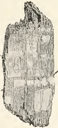
FIG. 10.—Medullary rays of oak-wood destroyed by Polyporus . The cells are still full of undissolved starch, hence appear white. (v. Tubeuf phot.)
