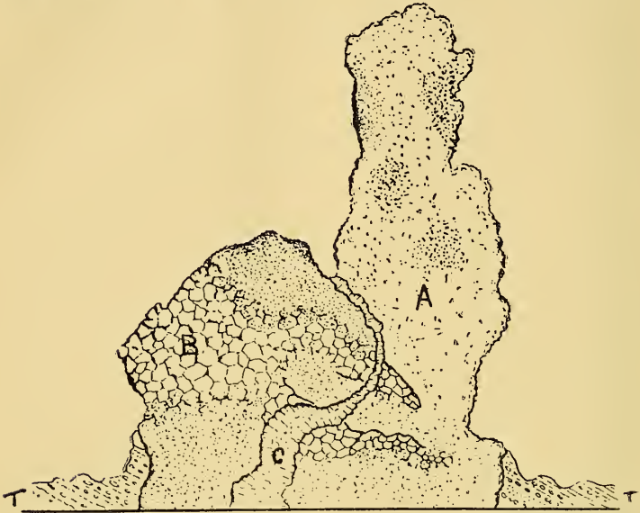
FIG. 1.—Diagram to illustrate structure of Rock and Spindle shore stack as seen from the east side. TT, older bedded tuffs of the vent forming the beach platform. A, intrusive basalt with included fragments. B, a portion of the basalt—forming the spindle—which, remaining clear of fragments, has jointed symmetrically. C, dyke cutting both A and B. Further references in text.
