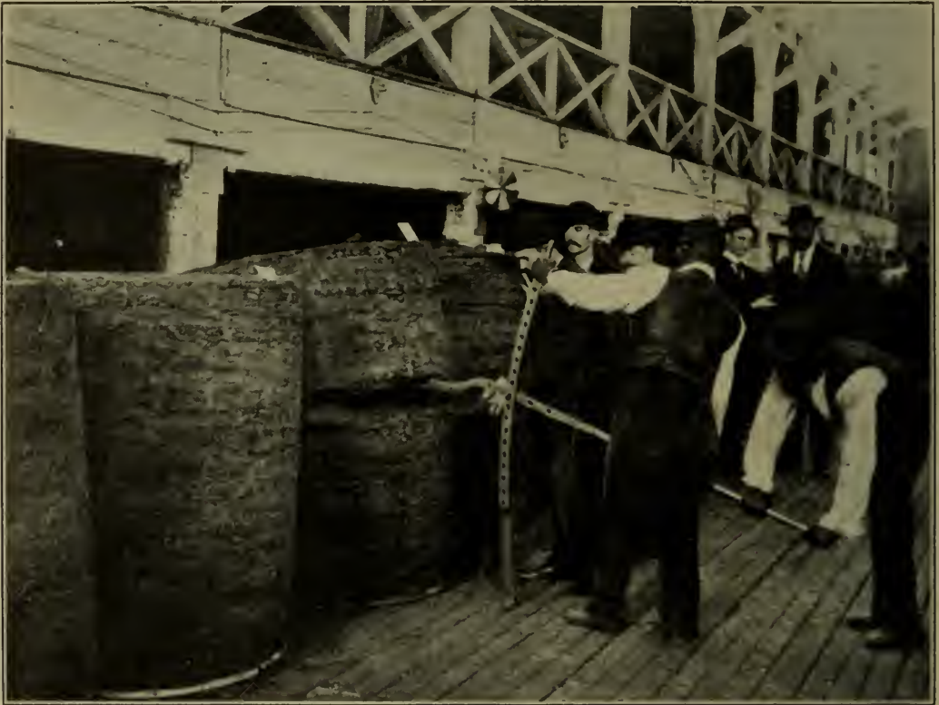
FIG. 8.—Breaking a hogshead and drawing a sample at a tobacco inspection, Louisville, Ky.
