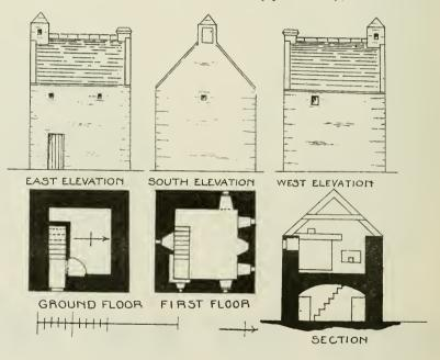
FIG. 1326 .- The Tower of Ardelach. Plans, Elevations, and Sections.
