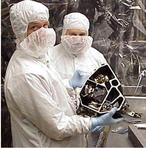
The Infrared Array Camera (IRAC) cryogenic assembly with top cover removed at NASA Goddard, Greenbelt, Maryland.
