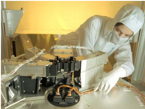
The Infrared Spectrograph (IRS) after integration with the Multiple Instrument Chamber at Ball Aerospace, Boulder, Colorado.
