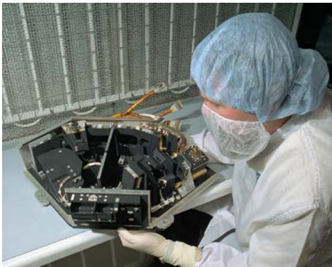
A Ball Aerospace technician holding the Multiband Imaging Photometer for SIRTf (MIPS) prior to integration (Ball Aerospace).
