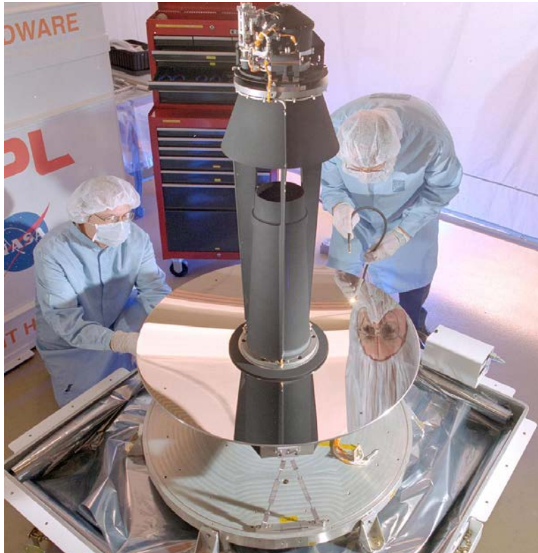
FIGURE 8.4. The beryllium mirror and telescope assembly at Ball Aerospace.
