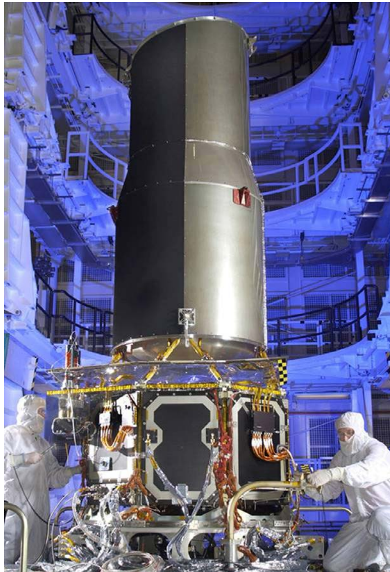
FIGURE 8.1. SIRTf during final integration and testing at Lockheed Martin, Sunnyvale, California (Russ Underwood, Lockheed Martin Space Systems).
