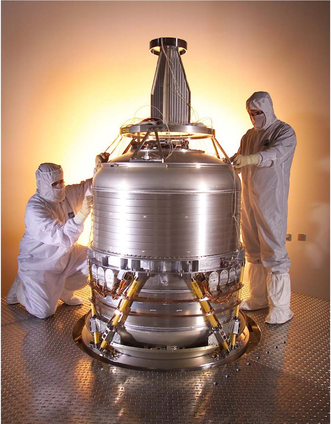
FIGURE 8.8. The instrument cryostat (with a mass model telescope on top), being prepared for shake testing.
