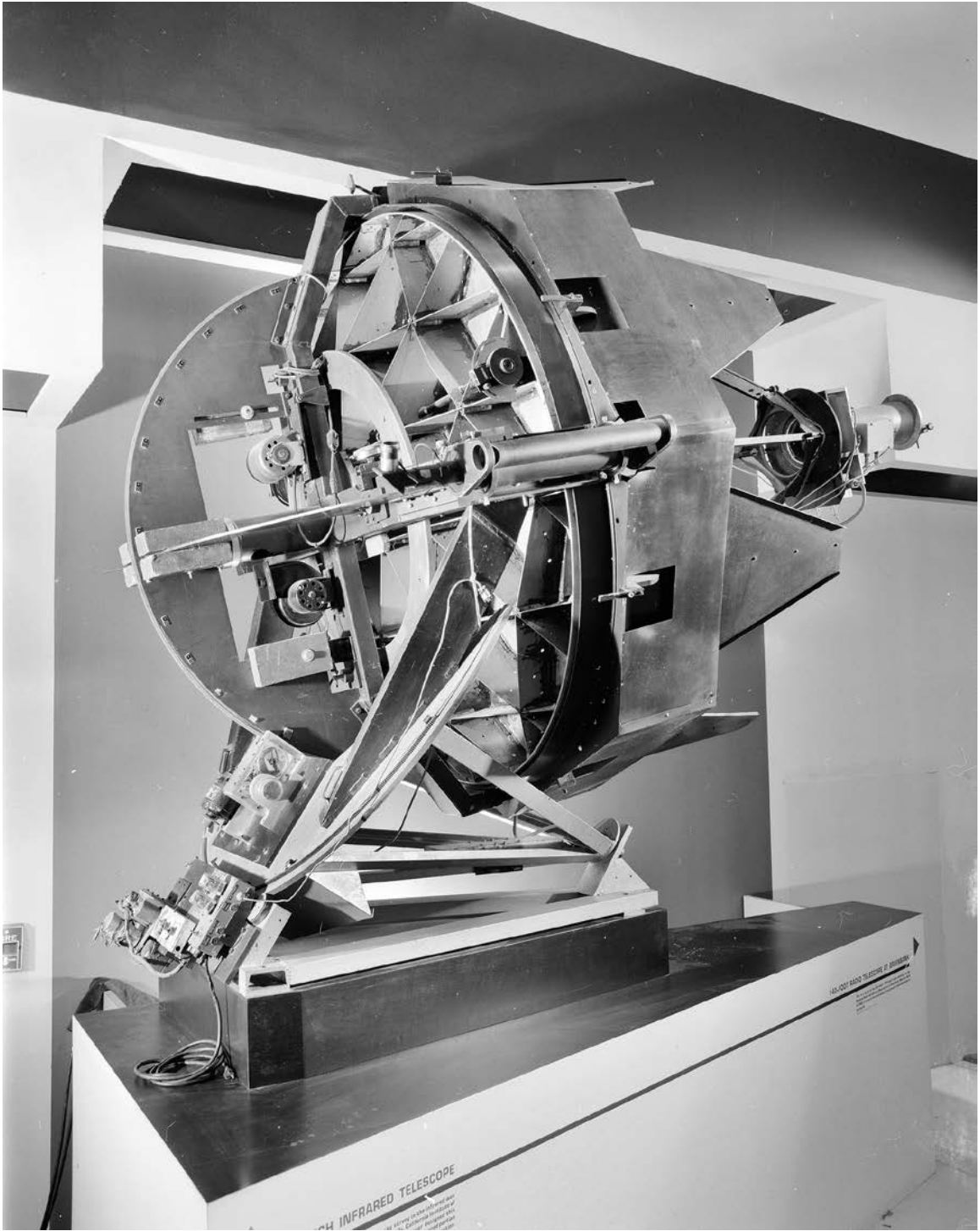
FIGURE 3.2. The 62-inch ground-based infrared telescope used for the Caltech Two-Micron Sky Survey (NASM).
