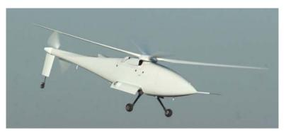
Figure 24: A-160 vertical take-off and landing (VTOL) unmanned air vehicle (UAV).
