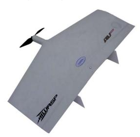
Figure 20: Wasp micro air vehicle.
